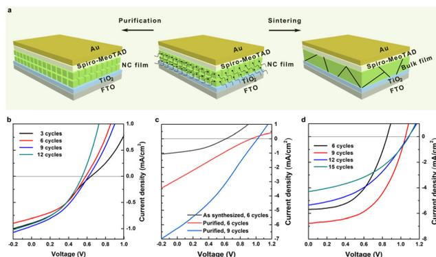
**Fig. 1** (a) Schematic showing the evolution of CsPbBr<sub>3</sub> solar cell structures after purification and sintering. (b–d) Current density–voltage curves of the CsPbBr<sub>3</sub> solar cells as a function of the deposition cycles measured under standard AM 1.5 conditions. Current density–voltage curves were recorded at a scan rate of 0.1 V s<sup>-1</sup> in the forward direction. (b) As-synthesized, (c) purified, (d) sintered.
