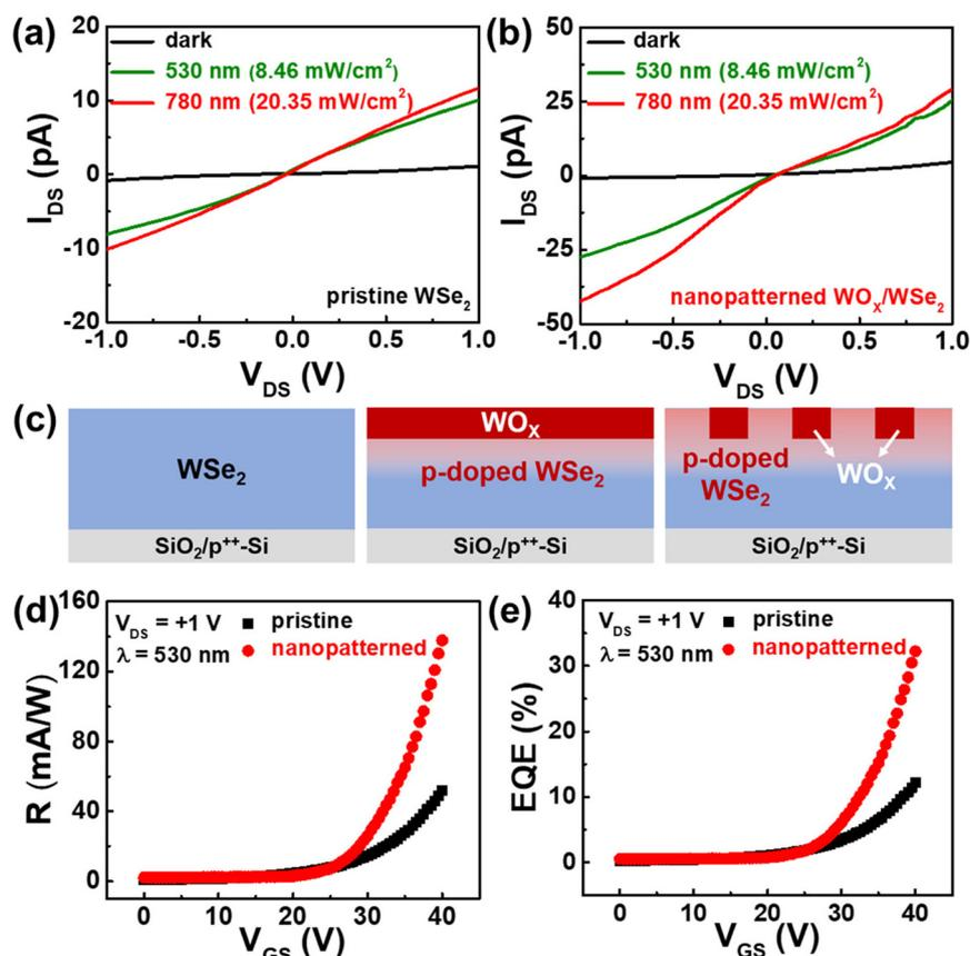
Fig. 3 Current-voltage characteristics of the (a) pristine and (b) nanopatterned WSe<sub>2</sub> device under different irradiation conditions (dark, and 530 nm and 780 nm wavelengths). (c) WSe<sub>2</sub> without a junction (left), WSe<sub>2</sub> with a planar junction (middle), and WSe<sub>2</sub> with a 3D nanostructured junction (right). (d) Responsivity (R) and (e) external quantum efficiency (EQE) at varying values of  $V_{GS}$ .
