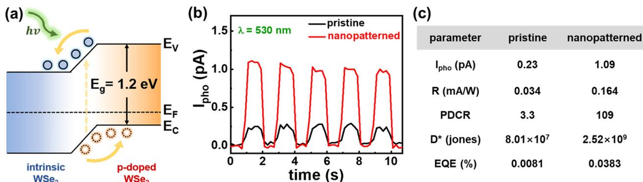
Fig. 5 (a) Mechanism of the self-powered WSe<sub>2</sub> photodetector. (b) Time-dependent photocurrent characteristics. (c) Optoelectronic performances of the pristine and nanopatterned WSe<sub>2</sub>.
