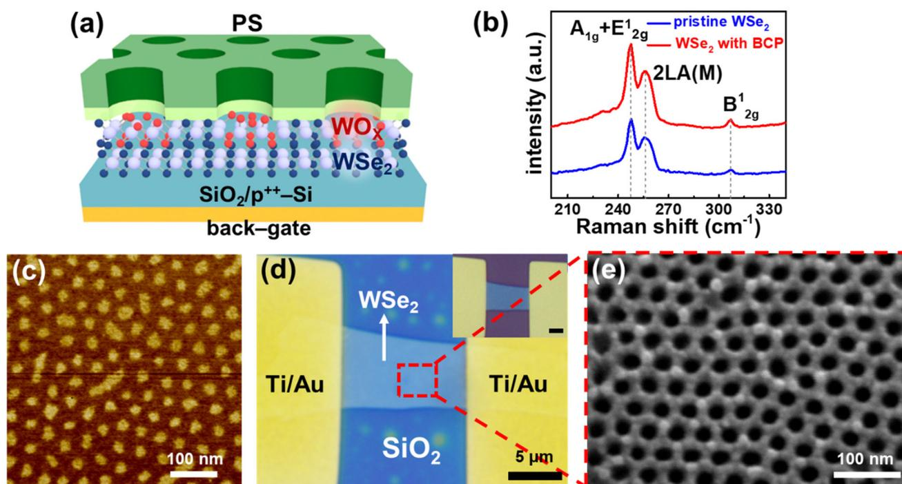
**Fig. 2** (a) Schematic of the 3D WSe<sub>2</sub> homojunction with nanoporous PS. (b) Micro-Raman spectra of the pristine and BCP-patterned WSe<sub>2</sub>. (c) AFM phase image of cylinder-forming PS-*b*-PMMA BCP thin films on the WSe<sub>2</sub> flake. (d) Optical microscopy of the WSe<sub>2</sub> photodetector. (e) SEM images of nanoporous BCP patterns on the WSe<sub>2</sub> photodetector.
