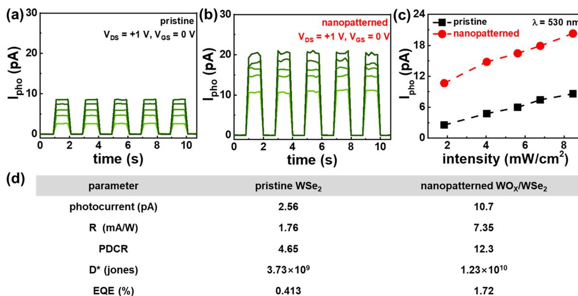
Fig. 4 Time-dependent photocurrent characteristics of the (a) pristine and (b) nanopatterned WSe<sub>2</sub> photodetector at varying optical intensities (530 nm wavelength). (c) Photocurrent at different optical intensities. (d) Optoelectronic parameters under the bias conditions of *V*<sub>DS</sub> = +1 V and *V*<sub>GS</sub> = 0 V considering the exposure of 530 nm with a light power density of 1.8 mW cm<sup>-2</sup>.
