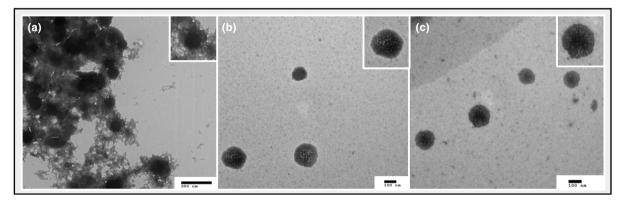
Fig. 7 Transmission Electron Microscopy (TEM) images (a) PEI-MAX/pDNA polyplexes at 1:1:2 pDNA ratio. Scale bar = 500 nm (b) NP10 nanogels at 1:1:2 pDNA ratio where the scale = 100 nm and (c) NP20 nanogels at 1:1:2 weight ratio where the scale bar = 100 nm.
