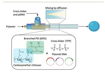
Fig. 2 Schematic of CFR demonstrating the smaller glass microcapillary delivering the carboxymethyl chitosan and branched PEI (CMC-bPEI) polymeric solution and the pAAV, pDG9 and PHGTI plasmids in solution with sodium tripolyphosphate as the cross-linker through the outer stream. The solutions mix by diffusion to form nanogels by ionic gelation.
