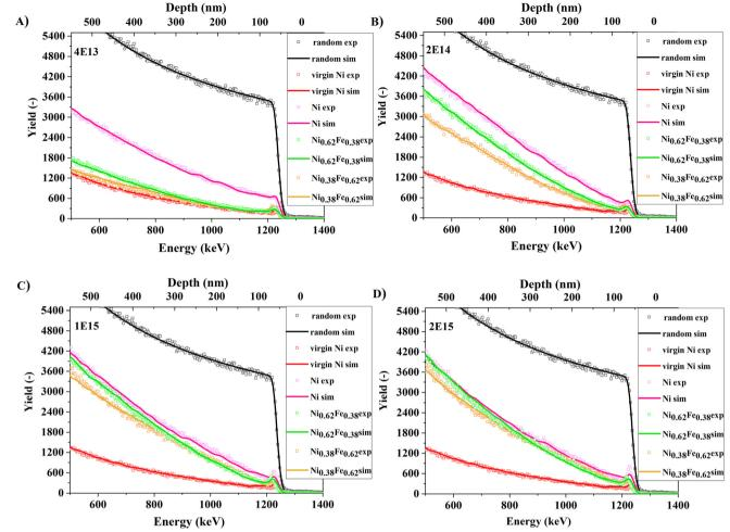
Fig. 3 Recorded ion channeling spectra of Ni, Ni<sub>0-62</sub>Fe<sub>0.38</sub> and Ni<sub>0-38</sub>Fe<sub>0.62</sub>. Specimens were irradiated with 1.5 MeV of Ni<sup>+</sup> at fluences of (A) 4  $\times$  10<sup>13</sup>, (B) 2  $\times$  10<sup>14</sup>, (C) 1  $\times$  10<sup>15</sup> and (D) 2  $\times$  10<sup>15</sup> ions per cm<sup>2</sup>. The intensities of the spectra were normalized to the highest Ni-random spectrum.
