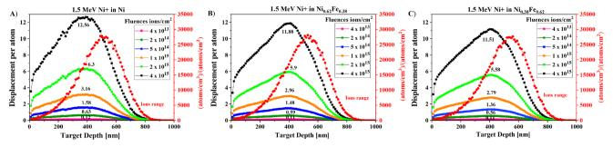
Fig. 1 Damage profiles of (A) Ni, (B) Ni<sub>0.62</sub>Fe<sub>0.38</sub> and (C) Ni<sub>0.38</sub>Fe<sub>0.62</sub> irradiated with 1.5 MeV of Ni<sup>+</sup> at fluences of  $4 \times 10^{13}$ ,  $2 \times 10^{4}$ ,  $5 \times 10^{14}$ ,  $1 \times 10^{15}$ ,  $2 \times 10^{15}$  and  $4 \times 10^{15}$  ions per cm<sup>2</sup>.
