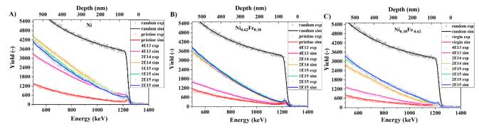
Fig. 2 Ion channeling spectra of (A) Ni, (B)  $Ni_{0.62}Fe_{0.38}$ , and (C)  $Ni_{0.38}Fe_{0.62}$  single crystals irradiated with fluences from  $4 \times 10^{13}$  to  $2 \times 10^{15}$  ions per cm<sup>2</sup>. Solid lines represent fits obtained using MC simulations. Virgin and random spectra are included as references.
