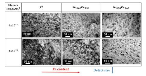
Fig. 8 TEM images of Ni, Ni<sub>0.62</sub>Fe<sub>0.38</sub>, and Ni<sub>0.38</sub>Fe<sub>0.62</sub> irradiated with fluences of  $4 \times 10^{13}$  ions per cm<sup>2</sup> and  $4 \times 10^{15}$  ions per cm<sup>2</sup>.
