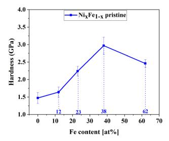
Fig. 4 Nanoindentation hardness of the non-irradiated fcc Ni and  $Ni_xFe_{1-x}$  single crystal alloys as a function of Fe content.
