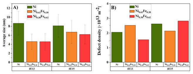
Fig. 9 (A) Average defect size calculated based on the TEM images and (B) defect densities of Ni, Ni<sub>0.62</sub>Fe<sub>0.38</sub>, and Ni<sub>0.58</sub>Fe<sub>0.62</sub> irradiated with fluences of  $4 \times 10^{13}$  ions per cm<sup>2</sup> and  $4 \times 10^{15}$  ions per cm<sup>2</sup>.
