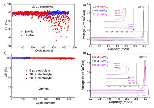
Fig. 4 Stability of Na plating and stripping on the Zn surface as a function of electrolyte volume, concentration and temperature: (a) faradaic efficiency of Zn//Na and Cu//Na cells using 20 µL of electrolyte; (b) efficiency of Zn//Na using gradually lowered electrolyte volumes; voltage profiles of the Zn//Na cell evaluated at (c) 25 and (d) 50 °C with 0.5, 1.0 and 2.0 M NaPF<sub>6</sub>. All cells were cycled at 2.0 mA cm<sup>-2</sup> and 3.0 mA h cm<sup>-2</sup>.
