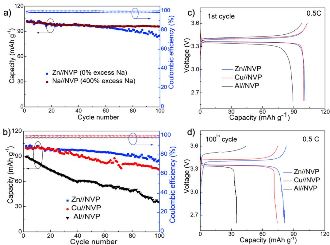
**Fig. 5** Electrochemical performance of anode-free Na metal full batteries: (a) capacity retention and CE of Zn//NVP and Na//NVP full cells; (b) capacity retention and CE of Zn//NVP, Cu//NVP, and Al//NVP anode-free cells; (c and d) charge/discharge voltage profiles of Zn//NVP, Cu//NVP, and Al//NVP anode-free cells for the 1<sup>st</sup> and 100<sup>th</sup> cycles.
