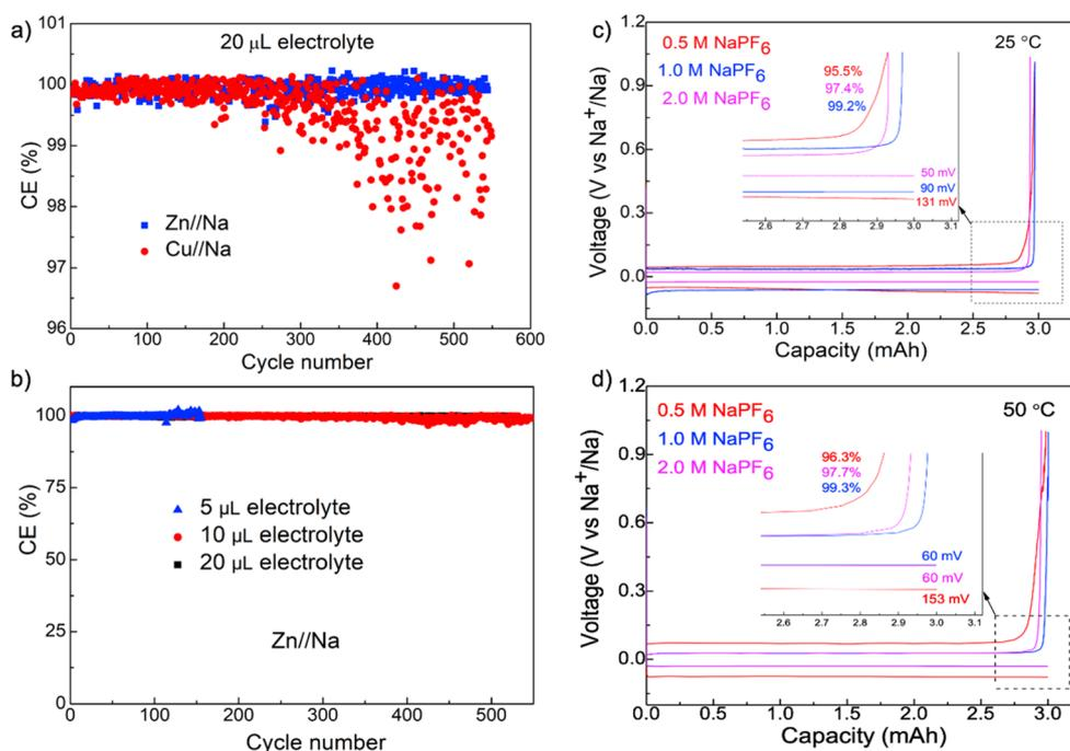
**Fig. 4** Stability of Na plating and stripping on the Zn surface as a function of electrolyte volume, concentration and temperature: (a) faradaic efficiency of Zn//Na and Cu//Na cells using 20  $\mu$ L of electrolyte; (b) efficiency of Zn//Na using gradually lowered electrolyte volumes; voltage profiles of the Zn//Na cell evaluated at (c) 25 and (d) 50 °C with 0.5, 1.0 and 2.0 M NaPF<sub>6</sub>. All cells were cycled at 2.0 mA cm<sup>-2</sup> and 3.0 mA h cm<sup>-2</sup>.
