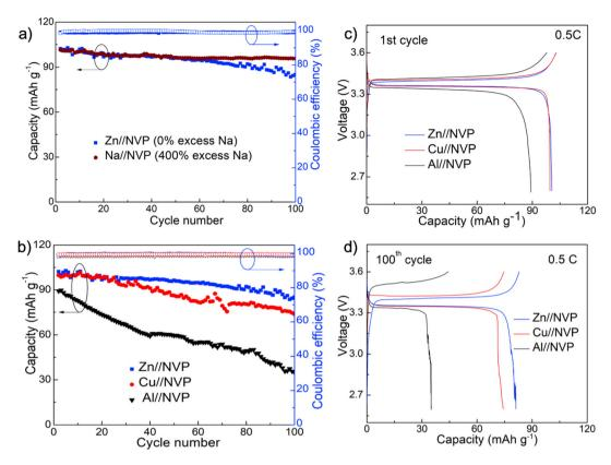
Fig. 5 Electrochemical performance of anode-free Na metal full batteries: (a) capacity retention and CE of Zn//NVP and Na//NVP full cells; (b) capacity retention and CE of Zn//NVP, Cu//NVP, and Al//NVP anode-free cells; (c and d) charge/discharge voltage profiles of Zn//NVP, Cu//NVP, and Al//NVP anode-free cells for the 1<sup>st</sup> and 100<sup>th</sup> cycles.
