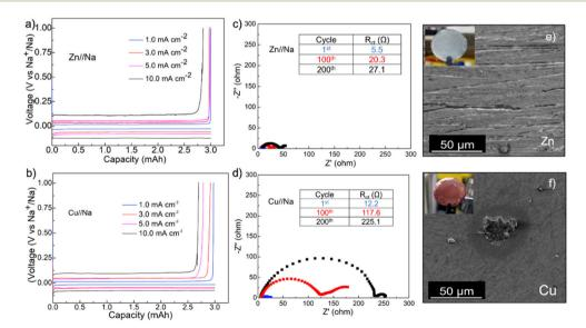
Fig. 3 Rate and cycling stability of Na plating and stripping in coin cells: voltage profiles at increasing current densities on (a) Zn and (b) Cu foils; Nyquist plots of (c) Zn//Na and (d) Cu//Na cells after 1, 100, and 200 cycles at 2.0 mA cm<sup>-2</sup>; SEM images and photographs (inset) of (e) Zn and (f) Cu foils after 200 cycles.
