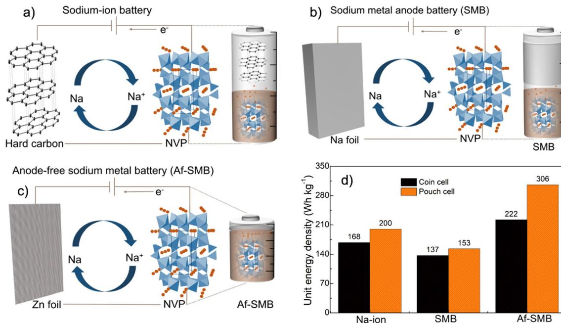
**Fig. 1** Schematic illustrations of different cell designs for Na batteries using NVP as the cathode material: (a) Na-ion batteries using the hard carbon anode; (b) Na metal full cells with the initial presence of Na metal in excess amount; (c) anode-free full cells with Zn foil current collectors; (d) estimated unit energy densities of these three cell designs with experimental data.
