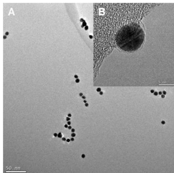
**Fig. 2** Representative TEM images of  $10 \mu\text{g ml}^{-1}$  10 nm AuNPs with  $4 \mu\text{g ml}^{-1}$  SP-B<sub>1-25</sub> and DPPC in 4 mM PB (DPPC/SP-B, 50 : 1 mol : mol), (A) taken at magnification 40 000× showing small agglomerates of the 10 nm AuNPs and (B) taken at magnification 500 000× showing crystalline structure of 10 nm AuNP and approximately 1 nm thick DPPC coating around the NP.
