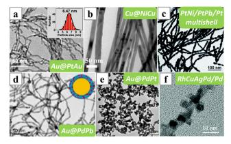
Fig. 18 TEM images of (a) Au@PtAu, (b) Cu@NiCu, (c) PtNi/PtPb/Pt, (d) Au@PdPb, (e) Au@PdPt core-shell or multishell nanowires and (f) RhCuAqPd/Pd nanowires synthesized depositing the alloy shell on the preformed metal nanowires. Reprinted with permission from ref. 146-151. Copyright 2021 from Science Press and Elsevier, 2017 from the Royal Society of Chemistry, 2020 from Springer Nature, 2017 from the American Chemical Society.
