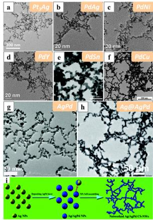
Fig. 15 TEM images of (a)  $Pt_3Ag$ , (b) PdAg, (c) PdNi, (d) PdY, (e) PdSn, (f) PdCu, (g) AgPd and (h) Ag@AgPd nanowires synthesized with PVP as the structure-directing reagent in aqueous solutions. (i) Schematics illustrating the oriented attachment of Ag@AgPd nanoparticles into networked Ag@AgPd nanowires. Reprinted with permission from ref. 127-129, 131, 133 and 134. Copyright 2020 from Springer Nature, 2018 and 2021 from the Royal Society of Chemistry, 2017 from Elsevier.
