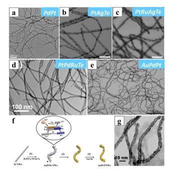
Fig. 23 TEM images of (a) PdPt, (b) PtAgTe, (c) PtRuAgTe, (d) PtPdRuTe and (e) AuPdPt nanowiress synthesized via replacing the Te nanowires with metal precursors. (f) Schematics illustrating the formation mechanism of AuPt porous nanowires and (g) the resulting TEM image of AuPt porous nanowires. Reprinted with permission from ref. 167, 169-171. Copyright 2019 from the Royal Society of Chemistry, copyright 2017, 2019 and 2022 from the American Chemical Society.
