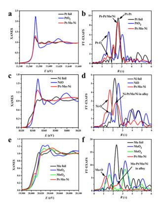
Fig. 2 XAS analyses of the PtMoNi NWs. XANES (a) and EXAFS (b) analysis of Pt L<sub>3</sub>-edge (FT range, 4.3 to 14.5 Å<sup>-1</sup>). XANES (c) and EXAFS (d) analysis of Ni K-edge (FT range, 2.5 to 12.5 Å<sup>-1</sup>). XANES (e) and EXAFS (f) analysis of Mo K-edge (FT range, 2.0 to 10.5 Å<sup>-1</sup>). Reprinted with permission from ref. 51. Copyright 2017 from AAAS.
