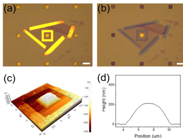
**Fig. 4** Optical micrographs of Au NPCs patterns (a) before and (b) after the KCN treatment. Scale bars indicate 10  $\mu\text{m}$ . (c) Atomic force microscopy image and (d) corresponding height profile of the device left under the reaction conditions for 3 h.
