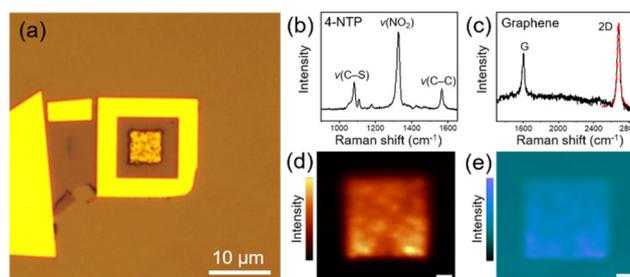
**Fig. 2** (a) Optical micrograph of a fabricated device. Raman spectra of (b) 4-NTP and (c) graphene taken at the center of the device. The red dashed curve in c shows the single Lorentzian fitting of the 2D band. Two-dimensional Raman mapping images of (d) the  $\nu(\text{NO}_2)$  peak of 4-NTP and (e) the 2D band of graphene measured inside the device. Scale bars indicate 1 μm.
