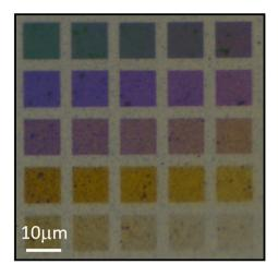
Fig. 6 Bright-field optical microscopy image of Mie resonators characterized by (L,q) geometric parameters in the range L(60 nm-100 nm)and q(60 nm - 100 nm).
