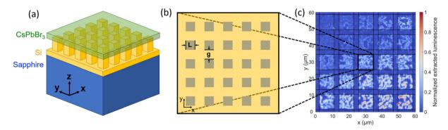
Fig. 1 (a) Schematic representation of the CsPbBr<sub>3</sub> layer deposited on Mie resonators, each corresponding to a set of (L,g) parameters. (b) Geometric parameters defining the size of the square pillars (L) and their side-to-side separation, which we refer to as the gap (q). (c) Perovskite luminescence, normalized to the maximum intensity of the image, over Mie resonators with varying (L,g) parameters.
