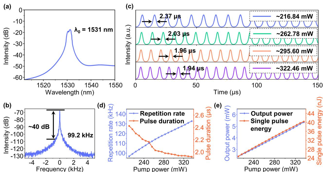
Fig. 6 (a) The optical spectrum and (b) RF spectrum over a 10 kHz span with a resolution bandwidth of 3 Hz at a pump power of 216.84 mW. (c) Temporal pulse trains under different pump powers. (d) Repetition rates and pulse durations *versus* the pump powers. (e) Output powers and single pulse energies *versus* the pump powers.  $\lambda_0$ : central wavelength.
