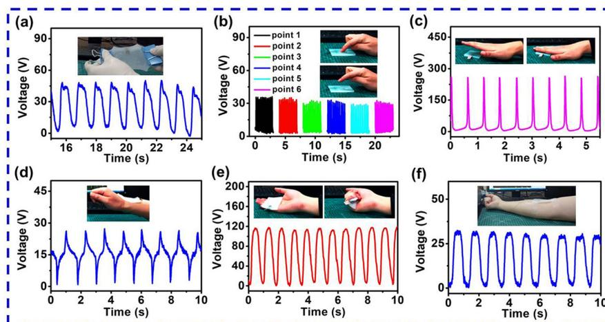
**Fig. 7** Demonstration of the MCH-TENG for harvesting human motion energy. (a) Stretching energy. (b) Finger press energy. (c) Hand tapping energy. (d) Wrist bending energy. (e) Hand gripping energy. (f) Elbow bending energy.
