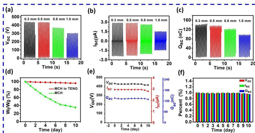
Fig. 5 The outputs of  $V_{oc}$  (a),  $I_{sc}$  (b) and  $Q_{sc}$  (c) of the MCH-TENGs with different thicknesses of silicone rubber. (d) Weight changes of the MCH in the MCH-TENG and open air as a function of storage time for 10 days. (e) Outputs and (f) retention rate of  $V_{oc}$ ,  $I_{sc}$  and  $Q_{sc}$  of the MCH-TENG as a function of storage time for 10 days.
