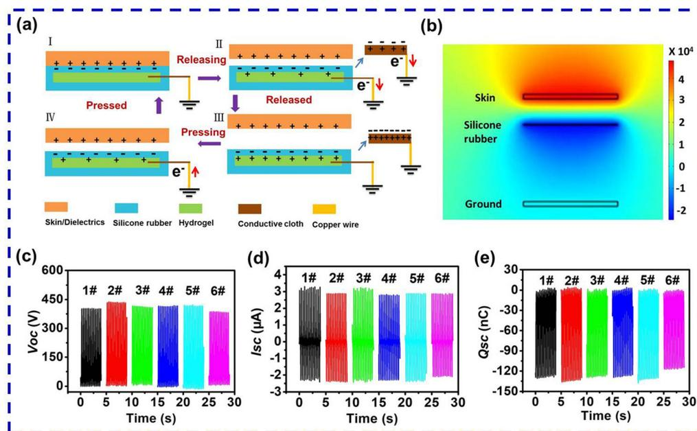
Fig. 2 Working mechanism and electrical performance of the MCH-TENG. (a) Schematic diagram of the working mechanism of the MCH-TENG. (b) Simulated potential distribution of the MCH-TENG. (c–e) Electrical outputs ( $V_{oc}$ ,  $I_{sc}$  and  $Q_{sc}$ ) of the 1#–6# MCH-TENGs.
