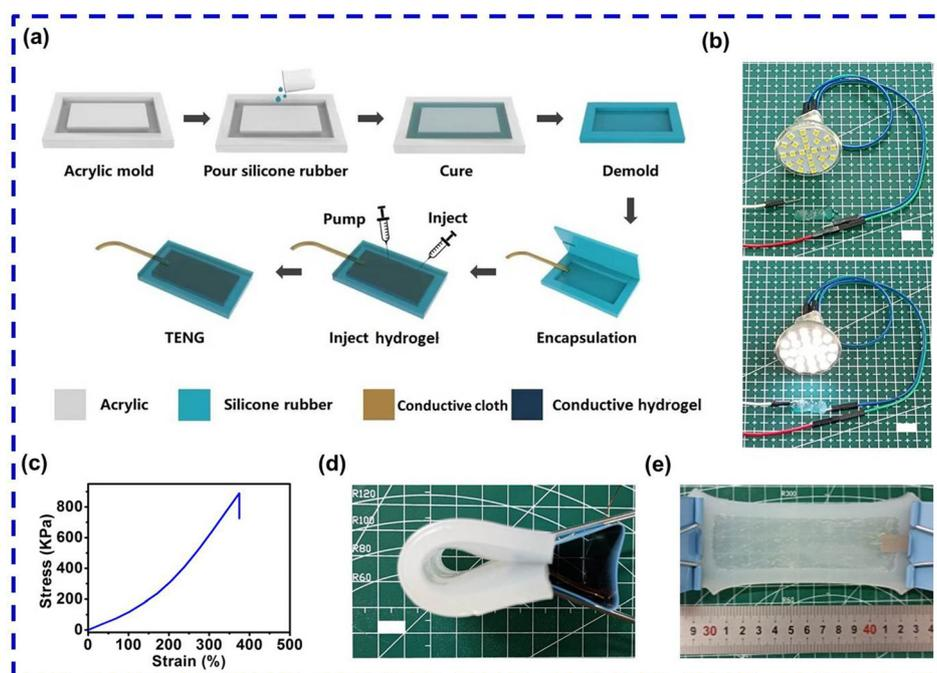
**Fig. 1** (a) Schematic diagram of the detailed fabrication process of the MCH-TENG. (b) Photographs of the circuit comprising of the MCH and LED light ( $V = 8 \text{ V}$ ; top: open circuit; bottom: closed circuit). (c) The stress–strain curve of the silicone rubber cube ( $59 \times 10 \times 2 \text{ mm}^3$ ). (d) and (e) Photographs of the MCH-TENG at bending (d) and stretching states (50%). (All scale bar = 1.0 cm.)
