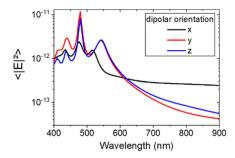
Fig. 8 Averaged simulated electric field intensity inside the Si blocks of the dimer plotted in a log scale for the x, y and z-oriented electric dipole source placed in between the dimer at a height of 90 nm. The dimer dimensions are W = 80 nm, L = 280 nm, H = 90 nm, and G = 10100 nm.
