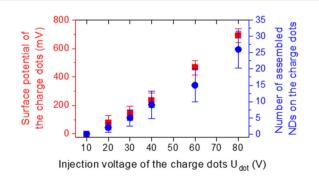
Fig. 3 Surface potential of the charge dots (left, red squares) and number of assembled NDs per charge dot (right, blue disks) as a function of the voltage amplitude  $U_{dot}$  used for charge dot injection.
