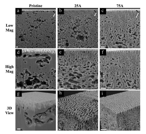
Fig. 3 (a-f) Cross-sectional SEM images and (g-i) reconstructed 3D volume of pristine membrane (a, d and g) and membrane modified with 3 cycles of AlO<sub>x</sub> SIS and 25 (b, e and h) or 75 cycles of AlO<sub>x</sub> ALD (c, f and i). Images d-f are higher magnifications of images a-c, respectively. The black arrows point to the highly ordered selective layer and the white arrows to the underneath supporting layer. All the scale bars are 200 nm.
