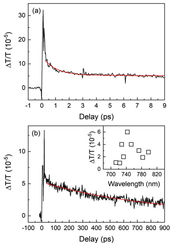
**Fig. 4** Dynamics of a room-temperature transient transmission at  $743 \pm 5$  nm. (a) Short time-scale measurement; (b) long time-scale measurement. The smooth red curves represent the fits. Inset: the amplitude spectrum of the slow component.
