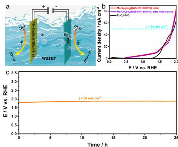
Fig. 5 (a) Schematic illustration of the electrocatalytic overall water splitting based on a Mo-Co<sub>9</sub>Se<sub>8</sub>@NiSe/NF-60||Pt/C couple. (b) LSV polarization curves of RuO<sub>2</sub>||Pt/C, initial Mo-Co<sub>9</sub>Se<sub>8</sub>@NiSe/NF-60||Pt/C, and Mo-Co<sub>9</sub>Se<sub>8</sub>@NiSe/NF-60||Pt/C after 1000 circles toward water electrolysis. (c) Long-term CP curve of the Mo-Co<sub>9</sub>Se<sub>8</sub>@NiSe/NF-60||Pt/C couple at 50 mA cm<sup>-2</sup>.
