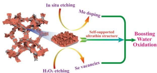
Fig. 6 Schematic illustration of the mechanism of OER activity based on Mo-Co<sub>9</sub>Se<sub>8</sub>@NiSe/NF-60.
