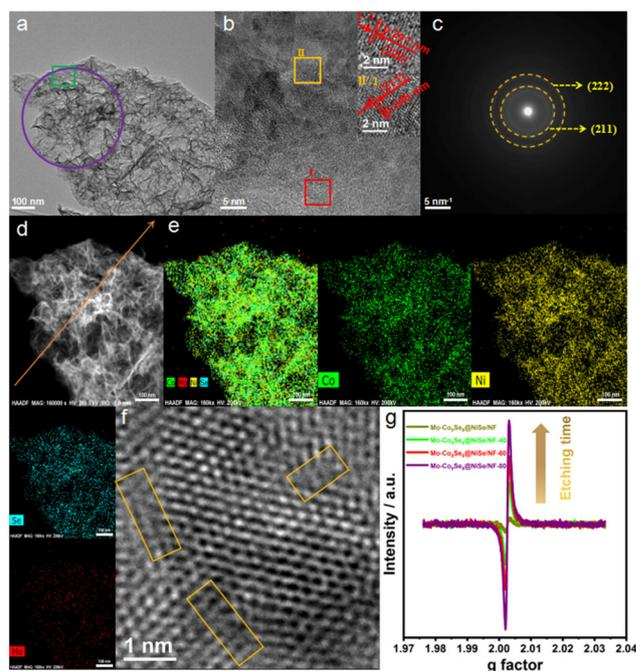
**Fig. 2** (a) TEM image, (b) HRTEM images (inset I-1 and II-2 correspond to the area of red square I and orange square II), (c) SAED patterns, (d) HAADF-STEM image, (e) EDX images, and (f) local HRTEM images of Mo-Co<sub>9</sub>Se<sub>8</sub>@NiSe/NF-60. (g) EPR spectra of etched Mo-Co<sub>9</sub>Se<sub>8</sub>@NiSe/NF with different etching durations compared to Mo-Co<sub>9</sub>Se<sub>8</sub>@NiSe/NF.
