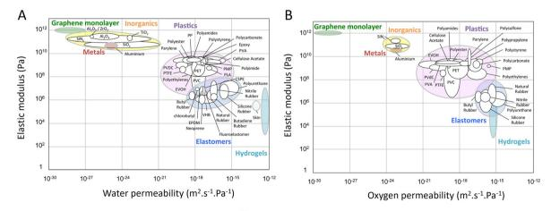
Fig. 6 The water and oxygen permeability of different materials.<sup>179</sup> Copyright 2018, American Chemical Society
