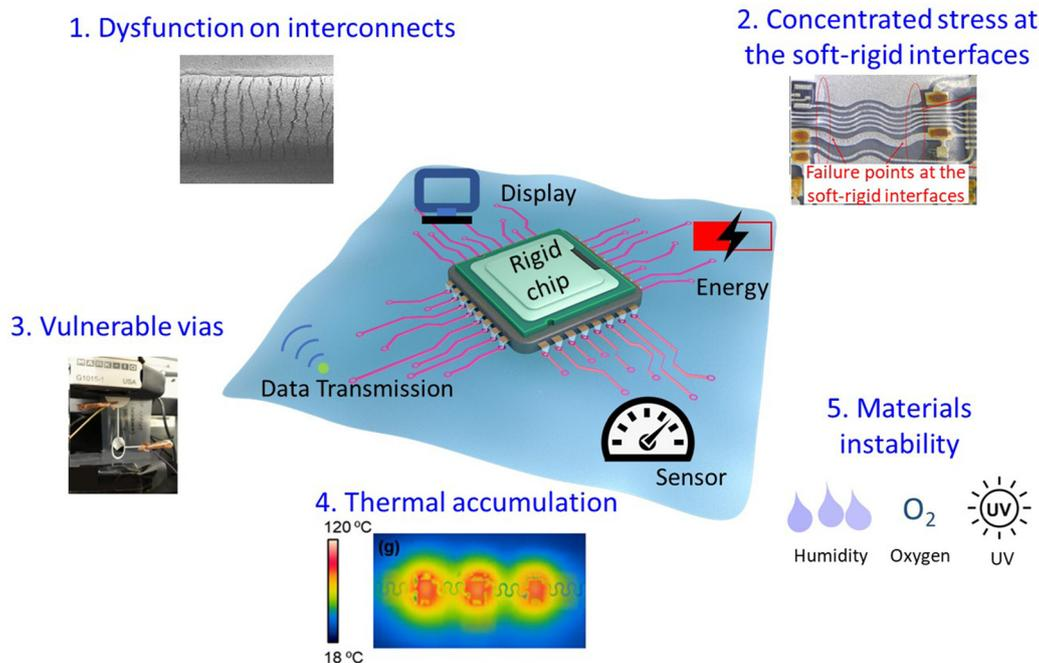
**Fig. 1** The common failure modes, including dysfunction on interconnects, concentrated stress on the soft-rigid interfaces, vulnerable vias, thermal accumulation and instability of stretchable materials (reproduced with permission,<sup>95</sup> copyright 2021, IEEE; reproduced with permission,<sup>111</sup> copyright 2020, Springer; reproduced with permission,<sup>116</sup> copyright 2021, Springer), and main components in printed stretchable electronics.
