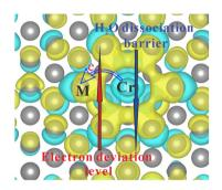
The effect of metal matrix M (M = Co, Ni, Cu) on the water dissociation performance of oxophilic Cr from density functional theory
