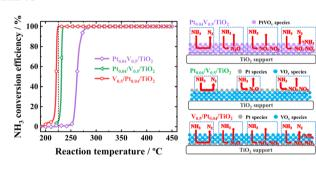
Influence of deposition order of dual active components on the NH<sub>3</sub>-SCO performance of the bimetallic Pt-V system supported on TiO<sub>2</sub>
