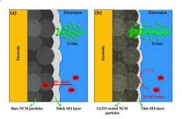
Li<sub>0.33</sub>La<sub>0.56</sub>TiO<sub>3</sub>, a novel coating to improve the electrochemical properties and safety of NCM523 cathode materials for Li-ion batteries
