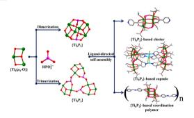
Ligand-directed structure evolution from a titanium-oxo cluster to coordination capsule and one-dimensional coordination polymer based on {Ti₃O} units
