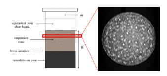
Formation and evolution of channels and voids in gravity sedimentation of kaolin suspensions studied by MRI
