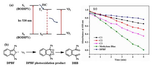
Fig. 9 (a) The mechanism of generation of singlet oxygen by brominated BODIPYs and (b) the degradation of DPBF in the presence of  ${}^{1}O_{2}$ ; (c) the plot of DPBF absorbance at 418 nm vs. irradiation time in the presence of meso-carbazole substituted BODIPY C1, and the brominated derivatives C2 and C3.
