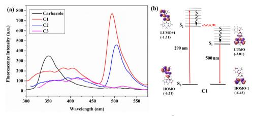
Fig. 5 (a) Fluorescence spectrum of meso-carbazole substituted BODIPYs C1, C2, and C3 ( $10^{-7}$  M,  $\lambda_{ex}$  = 290 nm) and carbazole ( $10^{-7}$  M) in chloroform at room temperature; (b) important molecular orbitals and electronic transitions occurring in C1 calculated using TDDFT at the M06/Def2-TZVPP//BP86/ Def2-TZVPP level of theory. Eigenvalues are given in eV.
