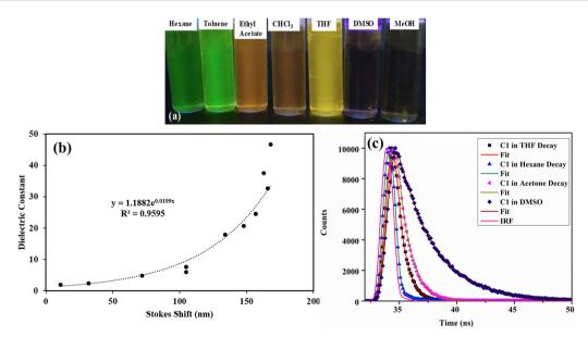
Fig. 7 (a) Photograph of **C1** in various solvents under UV irradiation-solvatochromism; (b) the plot of the dielectric constant vs. Stokes shift (nm) for **C1**; (c) the fluorescence decay profiles of **C1** in different solvents. The instrument response function (IRF) is shown in the red line.
