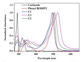
Fig. 2 Normalized absorption spectra of carbazole, phenyl-BODIPY, and meso-carbazole BODIPYs-C1, C2 and C3 in hexane ( $10^{-5}$  M) at room temperature
