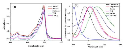
Fig. 6 (a) UV-visible spectrum ( $10^{-5}$  M) and (b) fluorescence spectrum ( $10^{-7}$  M,  $\lambda_{ex}$  = 480 nm) (normalized) of **C1** in various solvents at room temperature.
