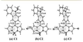
Fig. 3 Optimized geometry of meso-carbazole substituted BODIPY C1, C2, and C3 at the BP86/def2-TZVPP level of theory at the ground state in the gas phase. All angles are given in degrees and bond lengths in Å.
