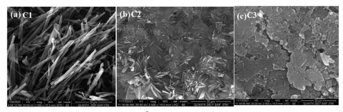
Fig. 12 SEM images of meso-carbazole substituted BODIPYs (10<sup>-5</sup> M) in DMSO-water mixtures (30/70 v/v): (a) C1; (b) C2; (c) C3; magnification: 2.5k, scale bar: 20 µm.
