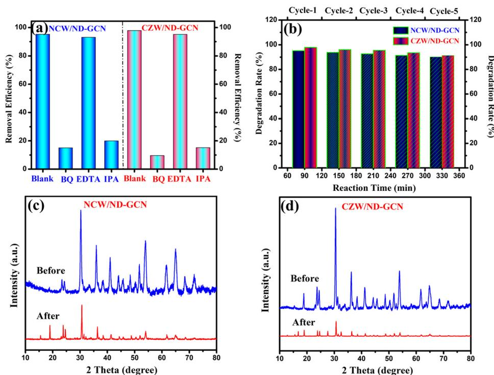
Fig. 12 (a) Radical scavenger investigations for pharmaceutical effluent degradation; (b) recycle stability test; (c) and (d) XRD spectra before and after the photocatalysis reaction.
