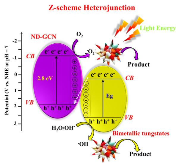
Scheme 1 Deciphering the Z-scheme charge transfer and degradation mechanism using NCW/ND-GCN and CZW/ND-GCN photocatalyst.
