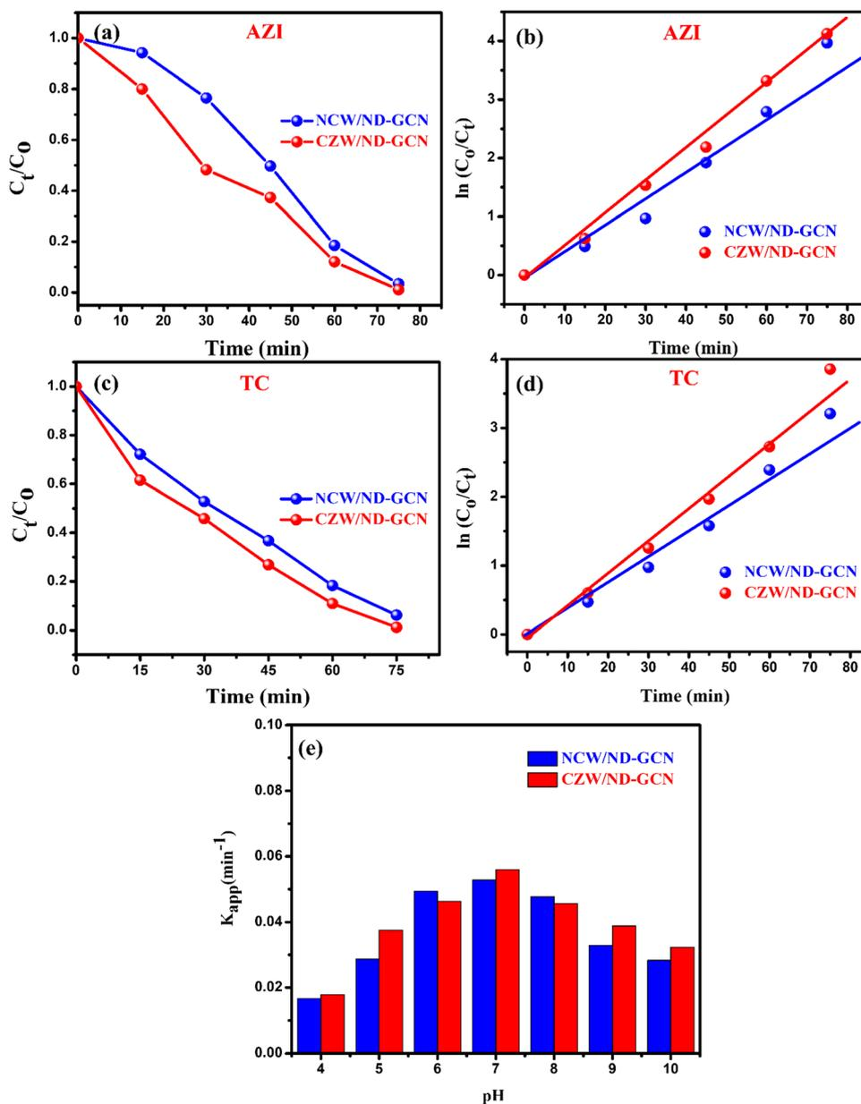
Fig. 10 (a) and (c)  $C_t/C_0$  plots; (b) and (d) linear fit of photocatalytic degradation of AZI and TC antibiotics and (e) effect of solution pH on the degradation of AZI over as-synthesized NCW/ND-GCN and CZW/ND-GCN photocatalyst.
