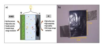
Fig. 8 (a) Schematic illustration of a hybrid supercapacitor with Ni-MOF as a positive electrode and activated carbon as a negative electrode in KOH aqueous electrolyte. (b) Digital photograph of the Ni-MOF//AC HSC device.
