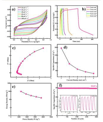
Fig. 9 (a) CV profile of HSC cell at different scan rates operated from 0 to 0.9 V. (b) GCD profiles for the HSC cell at different current rates (2-6 mA cm<sup>-2</sup>). (c) Nyquist plot of the HSC device. (d) Plot of the specific capacitance vs. current density. (e) Ragone plot for the HSC cell. (f) Cyclic durability test at a high current of 6 mA cm<sup>-2</sup> over 3000 GCD cycles; insets show the first and last five cycles.
