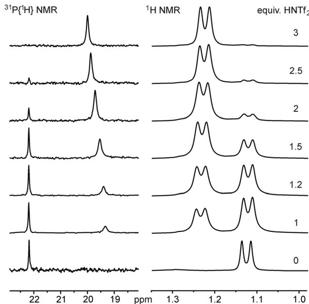
Fig. 5 Changes in the  $^{31}\text{P}\{^1\text{H}\}$  and  $^1\text{H}$  NMR spectra (region of  $\text{CHMe}_2$  protons) of complex 6 after adding various amounts of  $\text{HNTf}_2$  (recorded in  $\text{CDCl}_3$  at 25 °C). The amount of  $\text{HNTf}_2$  is given in molar equivalents per one gold atom.
