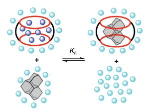
Fig. 2 Illustration of the changes in the solvation of the host and the guest that occur during the formation of CB[n]-quest complexes. Agua spheres, bulk water: Blue spheres, intracavity "high energy" water.
