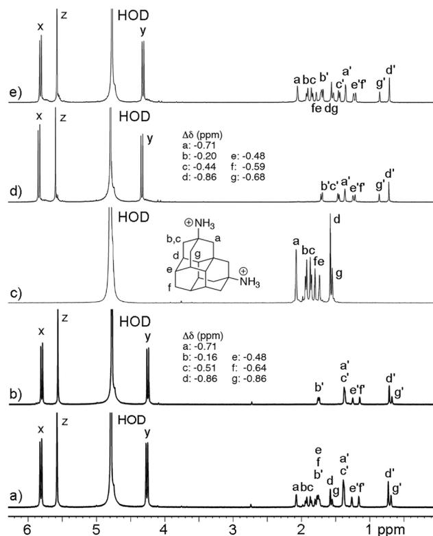
Fig. 4  $^1\text{H}$  NMR spectra recorded (600 MHz,  $\text{D}_2\text{O}$ ) for (a) a mixture of **G4** (2 mM) and CB[8] (1 mM), (b) a mixture of **G4** (1 mM) and CB[8] (1 mM), (c) **G4** (1 mM), (d) a mixture of **G4** (1 mM) and CB[7] (1 mM), and (e) a mixture of **G4** (2 mM) and CB[7] (1 mM). Resonances marked with primes (') arise from the host-**G4** complex.
