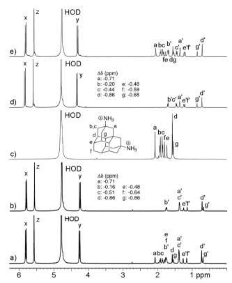
Fig. 4 <sup>1</sup>H NMR spectra recorded (600 MHz, D<sub>2</sub>O) for (a) a mixture of **G4** (2 mM) and CB[8] (1 mM), (b) a mixture of G4 (1 mM) and CB[8] (1 mM), (c) G4 (1 mM), (d) a mixture of G4 (1 mM) and CB[7] (1 mM), and (e) a mixture of G4 (2 mM) and CB[7] (1 mM). Resonances marked with primes (') arise from the host-G4 complex.
