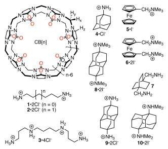
Structure of ultratight binding hosts CB[n] (n = 6, 7, 8) and selected Fig. 1
