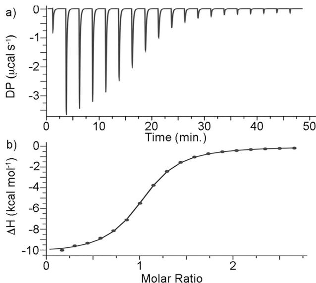
Fig. 6 (a) ITC thermogram recorded during the titration of CB[7] (145  $\mu\text{M}$ ) in the cell with guest **G1** in the syringe. (b) Fitting of the data to a 1 : 1 binding model with  $K_a = (1.6 \pm 0.1) \times 10^5 \text{ M}^{-1}$  and  $\Delta H = -10.4 \pm 0.076 \text{ kcal mol}^{-1}$ .
