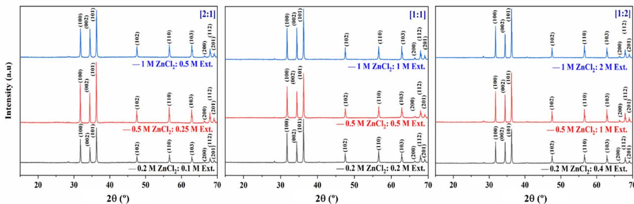
Fig. 1 XRD spectrum of the ZnO-NPs (JCPDS standard) synthesized using an eco-friendly *Phoenix dactylifera* L. extract in different ratios ([2 : 1], [1 : 1] and [1 : 2]) and concentrations (0.1, 0.2, 0.4, 0.5, 1 and 2 M).
