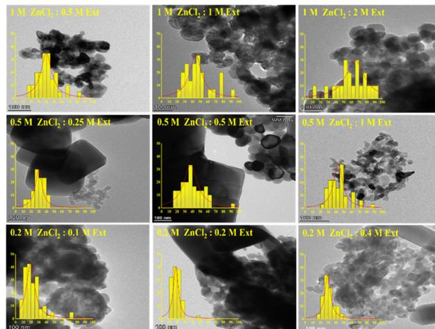
Fig. 3 Transmission electron microscopy (TEM) images of ZnO-NPs synthesized using an eco-friendly *Phoenix dactylifera* L. extract at different ratios ([2 : 1], [1 : 1] and [1 : 2]) and concentrations (0.1, 0.2, 0.4, 0.5, 1 and 2 M).
