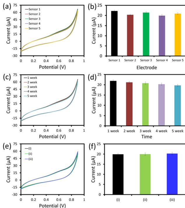
**Fig. 8** (a and b) The CV response of the 6  $\mu\text{L}$  cobalt oxide/SPCE sensor for 25  $\mu\text{M}$  UA for five similar fabricated sensors, (c and d) the CV response of 6  $\mu\text{L}$  cobalt oxide/SPCE sensor for 25  $\mu\text{M}$  UA for up to five weeks, and (e and f) the CV response of sensor in the presence of 0  $\mu\text{M}$  (i), 25  $\mu\text{M}$  (ii), and 50  $\mu\text{M}$  (iii) concentrations of each interferent with 25  $\mu\text{M}$  UA.
