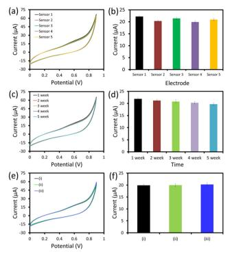
Fig. 8 (a and b) The CV response of the 6  $\mu$ L cobalt oxide/SPCE sensor for 25 μM UA for five similar fabricated sensors, (c and d) the CV response of  $6~\mu L$  cobalt oxide/SPCE sensor for 25  $\mu M$  UA for up to five weeks, and (e and f) the CV response of sensor in the presence of 0  $\mu$ M (i), 25  $\mu$ M (ii), and 50 µM (iii) concentrations of each interferent with 25 µM UA.
