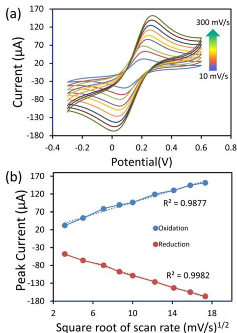
Fig. 6 (a) The CV responses of the best performing enzymeless sensor (6  $\mu\text{L}$  cobalt oxide/SPCE) in a probe solution at different scan rates (10–300  $\text{mV s}^{-1}$ ), and (b) the oxidation and reduction plot of the square root of the scan rate ( $\text{mV s}^{-1}$ )<sup>1/2</sup> vs. the redox peak current.
