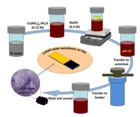
Fig. 1 A schematic illustration of the hexagonal shaped cobalt oxide nanosheet synthesis procedure using a hydrothermal method, and the UA sensor fabrication.
