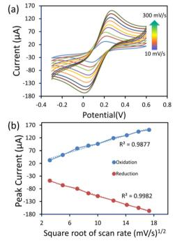
Fig. 6 (a) The CV responses of the best performing enzymeless sensor (6  $\mu L$  cobalt oxide/SPCE) in a probe solution at different scan rates  $(10-300 \text{ mV s}^{-1})$ , and (b) the oxidation and reduction plot of the square root of the scan rate (mV  $s^{-1}$ ) $^{1/2}$  vs. the redox peak current.
