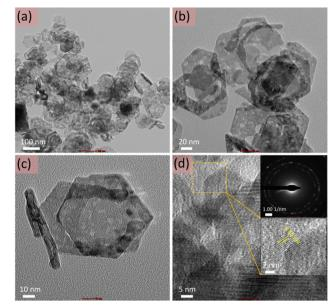
Fig. 3 The TEM images at different magnifications (a-c), and the HR-TEM (d) image of the hexagonal shaped cobalt oxide nanosheets. The insets in (d) are the SAED pattern (upper inset), and the magnified HR-TEM image (lower inset) of the hexagonal shaped cobalt oxide nanosheet.
