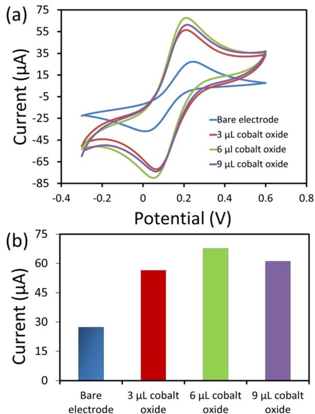
Fig. 5 (a) The CV responses of bare and cobalt oxide (3–9  $\mu\text{L}$ ) modified SPCE enzymeless UA sensors in 5 mM  $[\text{Fe}(\text{CN})_6]^{3-/4-}$  with a 0.1 M KCl redox probe solution (scan rate = 50  $\text{mV s}^{-1}$ ). (b) Histogram showing the peak current of bare and cobalt oxide nanosheet modified SPCE sensors.
