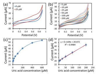
Fig. 7 (a) The CV response of the 6  $\mu L$  cobalt oxide/SPCE sensor in the absence (0  $\mu$ M) and presence (25  $\mu$ M) of UA in PBS buffer at a 50 mV s<sup>-1</sup> scan rate, (b) the CV response for different UA concentrations (5–400  $\mu$ M) in PBS buffer at a 50 mV  $\rm s^{-1}$  scan rate, (c) a plot showing oxidation current vs. UA concentration, and (d) calibrated linear range (5-200 µM) plot of the enzymeless sensor for three measurements.
