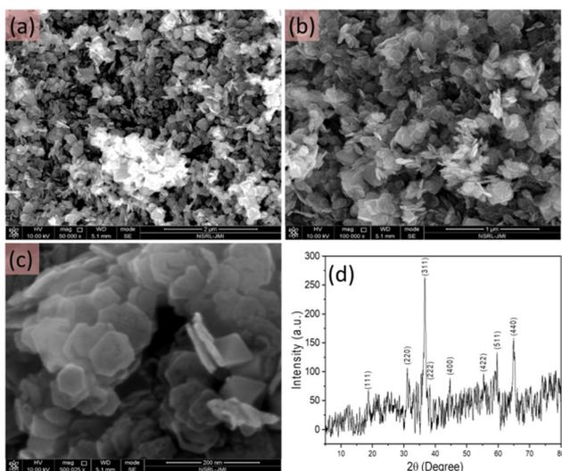
Fig. 2 FESEM images at different resolution (a–c) and the XRD pattern (d) of the as-synthesised hexagonal shaped cobalt oxide nanosheets.
