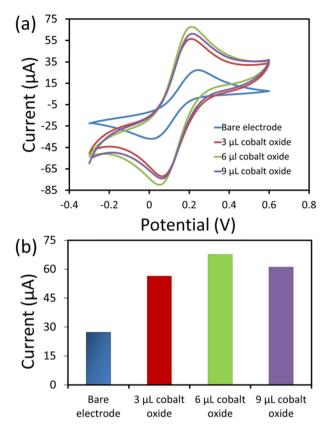
Fig. 5 (a) The CV responses of bare and cobalt oxide (3–9  $\mu$ L) modified SPCE enzymeless UA sensors in 5 mM  $\left[ \text{Fe(CN)}_6 \right]^{3-/4-}$  with a 0.1 M KCl redox probe solution (scan rate =  $50 \text{ mV s}^{-1}$ ). (b) Histogram showing the peak current of bare and cobalt oxide nanosheet modified SPCE sensors.
