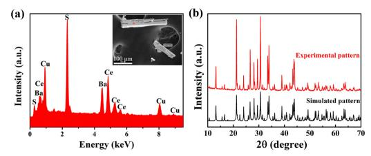
Fig. 1 (a) The EDX spectrum collected for a typical crystal of  $BaCeCuS_3$ . The inset of the figure shows an SEM picture of the  $BaCeCuS_3$  crystals. (b) The experimental PXRD pattern of the polycrystalline  $BaCeCuS_3$  sample, along with the corresponding simulated pattern obtained from the single crystal X-ray diffraction study.
