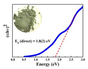
Fig. 4 The solid-state direct bandgap Tauc plot for the polycrystalline BaCeCuS<sub>3</sub> sample.
