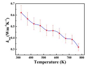
Fig. 5 The temperature-dependent total thermal conductivity  $(k_{tot})$  for the polycrystalline sample of BaCeCuS<sub>3</sub>.
