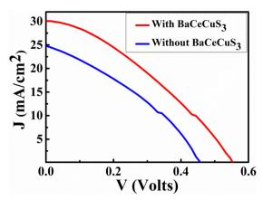
Fig. 7 The J vs. V plot of the FTO/TiO $_2$ /CdS/S $_n^2$ -/S $^2$ -/MWCNTs@Ni, and FTO/TiO<sub>2</sub>/CdS/BaCeCuS<sub>3</sub>/S<sub>n</sub><sup>2-</sup>/S<sup>2-</sup>/MWCNTs@Ni foam cell.
