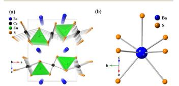
Fig. 2 (a) The unit cell structure of BaCeCuS<sub>3</sub> and (b) the Ba coordination
