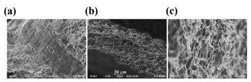
Fig. 6 The cross-sectional (a-c) FE-SEM images of the BaCeCuS<sub>3</sub> pellet used for the thermal conductivity measurements. The surface of the pellet is also visible in (b)
