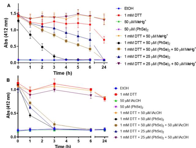
Fig. 4 Thiol oxidase activity of (PhSe)<sub>2</sub> and its inhibition by (A) MeHg<sup>+</sup> and (B) IAcOH. The lines and symbols for MeHg<sup>+</sup> (green) or (PhSe)<sub>2</sub> (purple) are harder to be visualized because they are almost coincident with that of EtOH (dark-blue).
