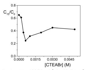
Fig. 4 Photodegradation of OG ( $2.0 \times 10^{-4}$  M) by TiO<sub>2</sub> (0.4 g L<sup>-1</sup>) in an aqueous dispersion at pH 12 after 15 min of irradiation (12 UV lamps) as a function of CTEABr concentration;  $\lambda_{anal}$  = 498 nm.
