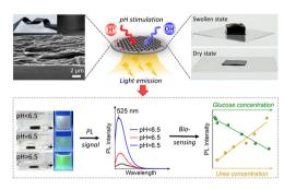
A nanofluidic sensing platform based on robust and flexible graphene oxide/chitosan nanochannel membranes for glucose and urea detection
