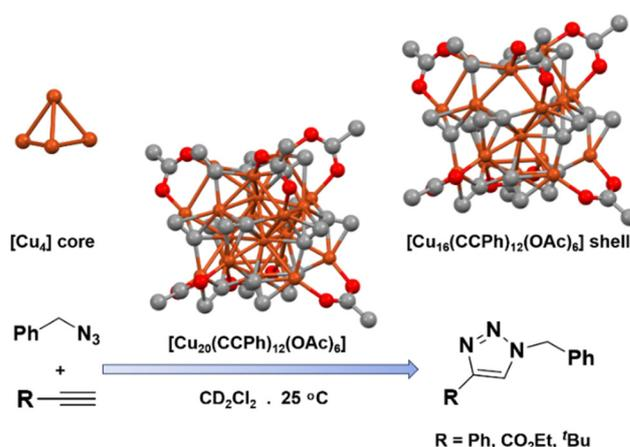
**Fig. 4** Structural architecture of [Cu<sub>20</sub>(CCPh)<sub>12</sub>(OAc)<sub>6</sub>] NC and its effectiveness towards [3+2] cycloaddition reaction. Cu displayed in brown color; O displayed in red color and C displayed in light dark color. Other ligands were removed for clarity. Figure created based on the cif file deposition of ref. 66.
