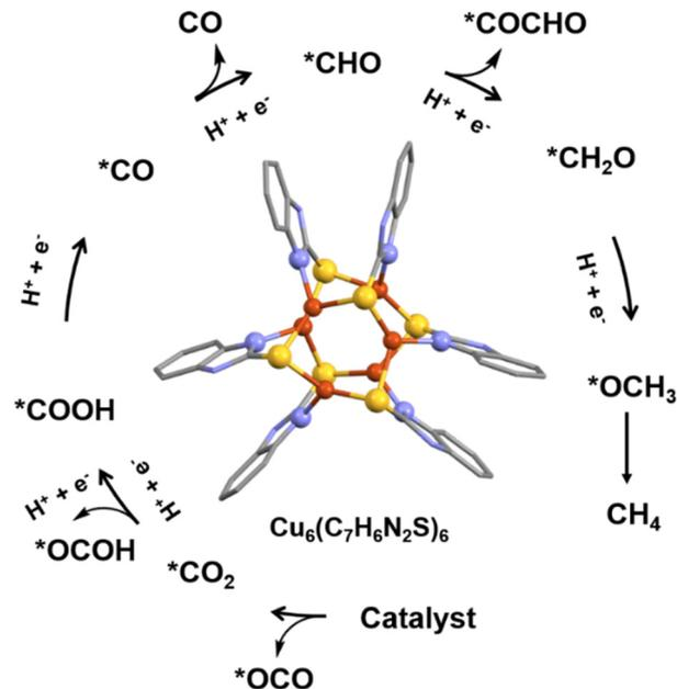
Fig. 10 Effect of the structural architecture and the specific combinatorial active sites for the selective  $\text{CO}_2$ RR product formation. Cu displayed in brown color; S displayed in yellow color; N displayed in blue color and C displayed in light dark color. Other ligands were removed for clarity. Figure created based on the cif file deposition of ref. 83.
