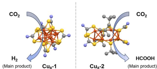
Fig. 9 Effect of the structural architecture of  $\text{Cu}_8$  NC in selectivity of  $\text{CO}_2$ RR product formation. Cu displayed in brown color; S displayed in yellow color; N displayed in blue color and C displayed in light dark color. Other ligands were removed for clarity. Figure created based on the cif file deposition of ref. 81.
