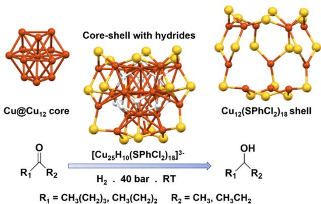
Fig. 2 Structural architecture of  $[\text{Cu}_{25}\text{H}_{10}(\text{SPhCl}_2)_{18}]^{3-}$  NC and its effectiveness towards hydrogenation reaction. Cu displayed in brown color; S displayed in yellow color and H displayed in white color. Other ligands were removed for clarity. Figure created based on the cif file deposition of ref. 61.
