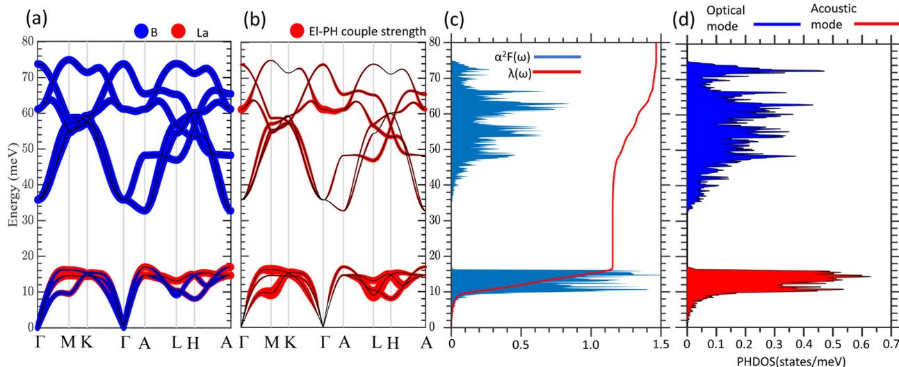
**Fig. 2** LaB<sub>2</sub> phonon related properties. (a) Phonon dispersion with atom resolved contributions. The size of the colored spheres illustrate the atomic contributions. (b) Phonon dispersion with EPC strength  $\lambda_{qv}$  indicated by the size of red spheres. (c) Eliashberg function  $\alpha^2F(\omega)$  and integrated Eliashberg function  $\lambda(\omega)$ . (d) Phonon density of states (PHDOS).
