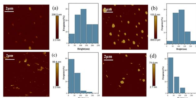
Fig. 3 AFM images and statistical size distribution of few-layer NbSe<sub>2</sub>/Nb<sub>2</sub>O<sub>5</sub> nanosheets under the centrifugation speed of (a) 1000 rpm, (b) 3000 rpm, (c) 5000 rpm, and (d) 7000 rpm.
