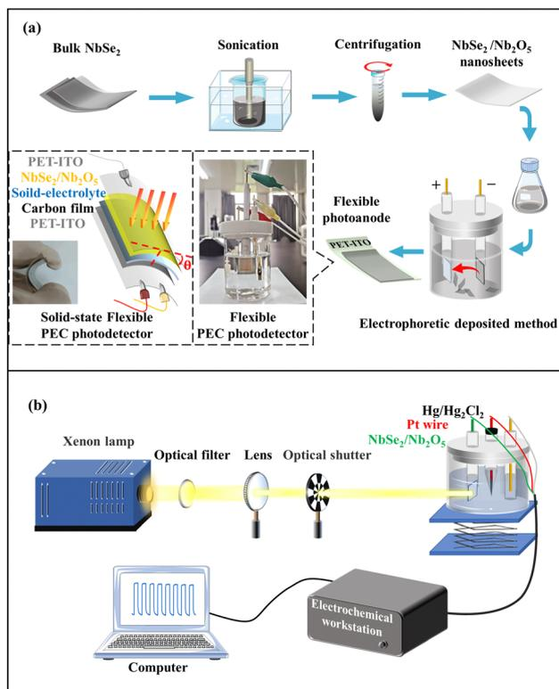
Fig. 1 (a) The preparation of the NbSe<sub>2</sub>/Nb<sub>2</sub>O<sub>5</sub>-based PEC photodetector and solid-state PEC photodetector, and (b) photoelectric performance measurement.
