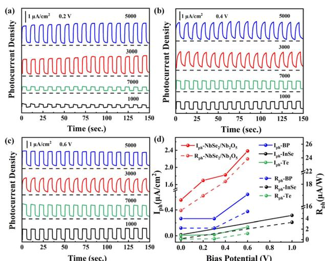
Fig. 5 Time-dependent photocurrent density of NbSe<sub>2</sub>/Nb<sub>2</sub>O<sub>5</sub> under the different centrifugal speed (1000, 3000, 5000, and 7000 rpm)-based PEC photodetectors was measured at (a) 0.2 V, (b) 0.4 V, and (c) 0.6 V; (d)  $I_{ph}$  and  $R_{ph}$  values of the 2D material-based PEC-type photodetector, including NbSe<sub>2</sub>/Nb<sub>2</sub>O<sub>5</sub> (this work), BP,<sup>41</sup> InSe,<sup>43</sup> and Te.<sup>42</sup>
