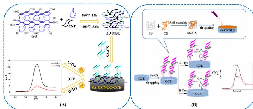
Fig. 8 (A) Diagram of the construction of the SA-CS-NGC/GCE chiral sensing platform.<sup>172</sup> Reprinted from X. Niu *et al.*, *Bioelectrochemistry*, 2020, **131**, 1–11 Copyright (2020), with permission from Elsevier. (B) The preparation of SS-CS/GCE and the proposed mechanism for the chiral electrochemical recognition of Tyr enantiomers on SS-CS/GCE.<sup>173</sup> Reprinted from J. Zou *et al.*, *Talanta*, 2019, **195**, 628–637 Copyright (2019), with permission from Elsevier.
