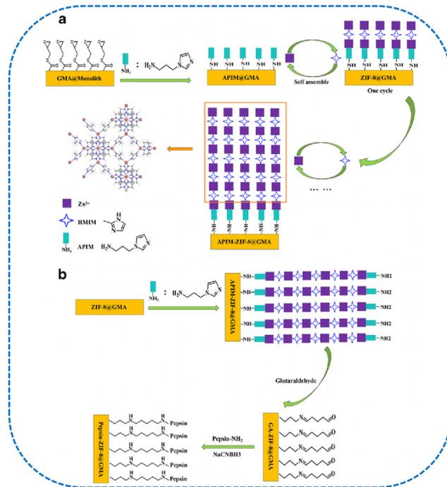
Fig. 10 (a) Scheme for the preparation of ZIF-8@GMA monolithic column and (b) Pepsin-ZIF-8@GMA monolithic column.<sup>182</sup> Reprinted from W. Ding *et al.*, *Microchimica Acta*, 2020, **187**, 1–10 Copyright (2020), with permission from Springer Nature.
