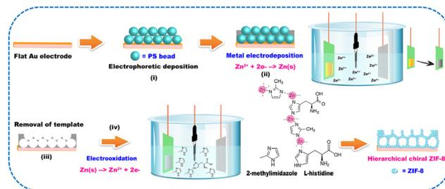
**Fig. 6** Illustration of the synthesis steps of hierarchical macroporous chiral ZIF-8, including (i) PS bead assembly *via* electrophoretic deposition, (ii) electrodeposition of macroporous Zn, (iii) removal of PS beads, and (iv) electrooxidation of Zn in the presence of organic ligands.<sup>131</sup> Reprinted from D. Suttipat *et al.*, *ACS Appl. Mater. Interfaces*, 2020, **12**, 36548–36557 Copyright (2020), with permission from American Chemical Society.
