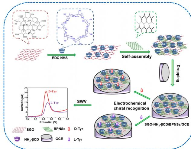
Fig. 7 Preparation of a chiral sensor SGO- $\text{NH}_2$ - $\beta$ -CD/BPNSs/GCE for the electrochemical recognition of Tyr enantiomers.<sup>141</sup> Reprinted from J. Zou *et al.*, *ACS Appl. Nano Mater.*, 2021, **4**, 13329–13338 Copyright (2021), with permission from American Chemical Society.
