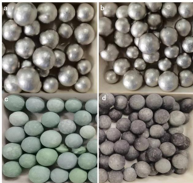
Fig. 2 Appearance of (a) fresh and (b) used Ir/Ni. Appearance of (c) fresh and (d) used Ir-Ni/Al<sub>2</sub>O<sub>3</sub> catalysts.
