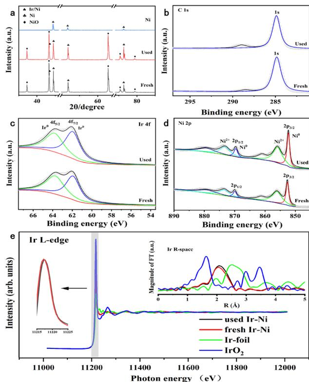
Fig. 4 (a) XRD patterns for Ni and fresh and used Ir/Ni samples. (b–d) Ni 2p, Ir 4f, and C 1s XPS spectra of fresh and used Ir/Ni. (e) XANES spectra of the Ir  $L_{3}$ -edge from the Ir/Ni catalyst, with Ir foil and  $\text{IrO}_2$  as references. Inset: Ir  $L_{3}$ -edge EXAFS in R space from the Ir/Ni catalyst, with Ir foil and  $\text{IrO}_2$  as references.
