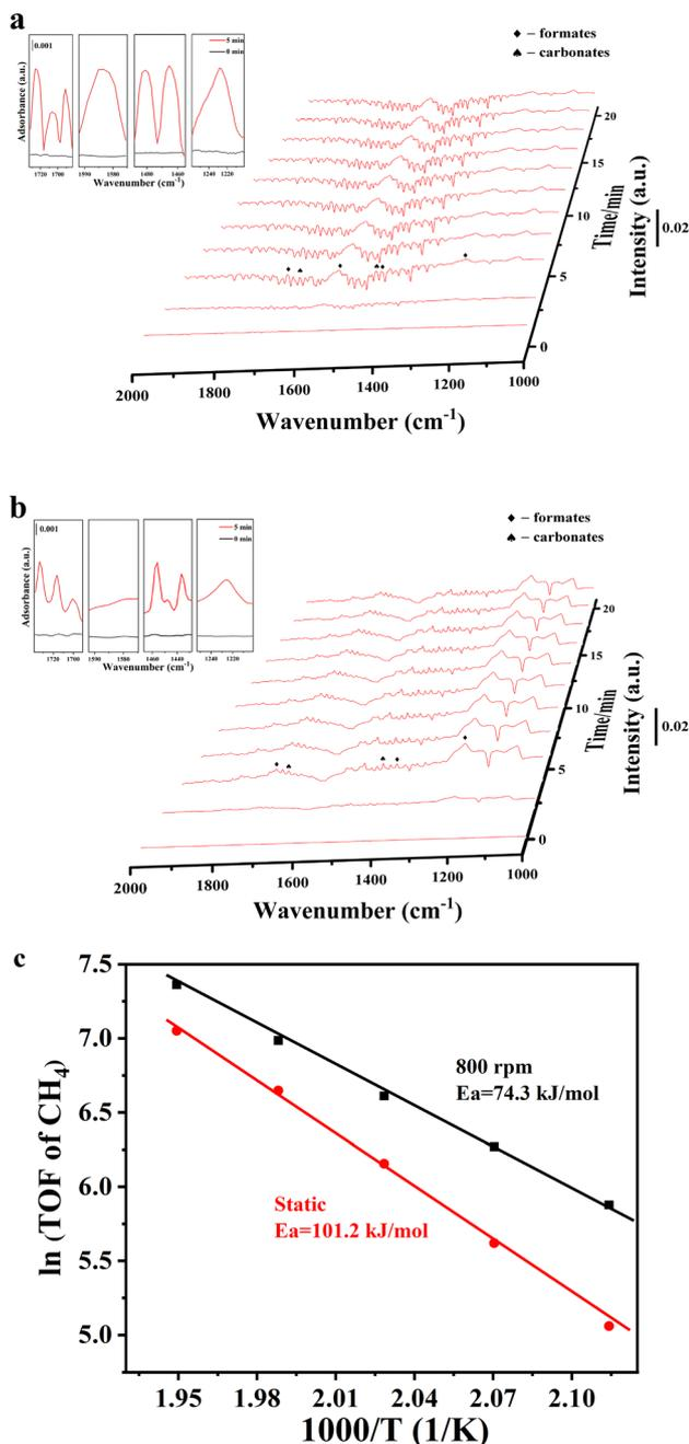
Fig. 6 *In situ* DRIFTS studies of CO<sub>2</sub> + H<sub>2</sub> over (a) Ir/Ni and (b) Ni catalysts under 150 °C. (c) The apparent activation energy from a kinetic activity test.
