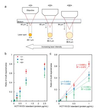
(a) Schematic diagram of the relationship between the focusing distance (FD) and the laser spot diameter at the bottom of the microchannel. (b and c) The ratio of the multi-layered area at each FD. Error bars present the standard deviations (n = 3). The assembly area and multilayered area at each FD are presented in Fig. S5 of the ESI.†
