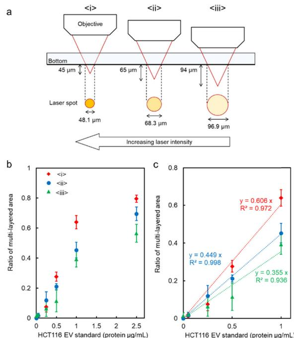
**Fig. 4** (a) Schematic diagram of the relationship between the focusing distance (FD) and the laser spot diameter at the bottom of the microchannel. (b and c) The ratio of the multi-layered area at each FD. Error bars present the standard deviations ( $n = 3$ ). The assembly area and multi-layered area at each FD are presented in Fig. S5 of the ESI.†
