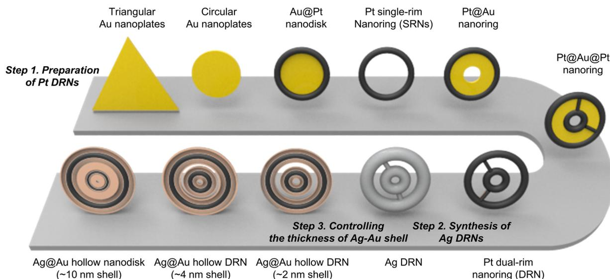
**Fig. 1** Schematic illustration of the synthetic pathway of Ag–Au alloy DRNs. To synthesize Ag–Au alloy DRNs, multiple synthetic chemical steps are employed, including selective Pt deposition, inner Au etching, and concentric growth of Au onto Pt skeletons.
