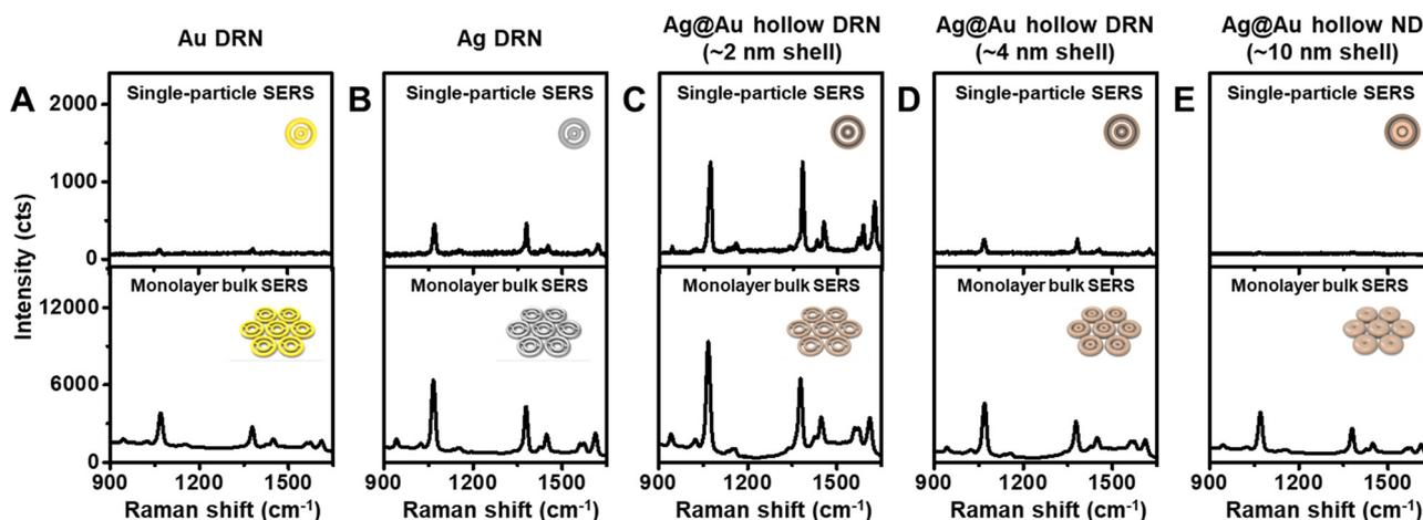
Fig. 3 Single-particle SERS and bulk SERS measurements. Single-particle SERS spectra and bulk SERS spectra of (A) Au DRNs, (B) Ag DRNs, (C) Ag@Au hollow DRNs (the thickness of Ag–Au shell:  $\sim 2$  nm), (D) Ag@Au hollow DRNs (the thickness of Ag–Au shell:  $\sim 4$  nm), and (E) Ag@Au hollow nanodisks (the thickness of Ag–Au shell:  $\sim 10$  nm).
