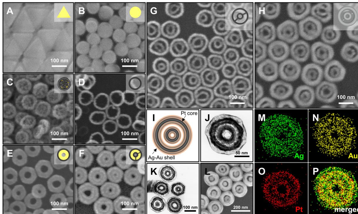
**Fig. 2** Morphological evolution of bimetallic alloy Ag@Au hollow dual-rim nanorings (DRNs) using multi stepwise chemical reactions. FE-SEM images of (A) triangular Au nanoplates, (B) circular Au nanoplates, (C) Au@Pt nanodisks, (D) Pt single-rim nanorings, (E) Pt@Au nanorings, (F) Pt@Au@Pt nanorings, (G) Pt DRNs, and (H) Ag DRNs. (I–L) A schematic illustration, TEM images and an FE-SEM image of Ag@Au hollow DRNs. (M–P) EDS mapping images of an Ag@Au hollow DRN.
