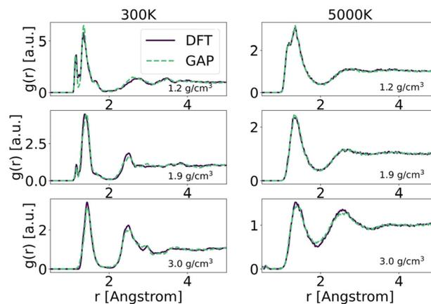
Fig. 1 Radial distribution functions of atomistic samples generated *via* the quenching from the melt protocol using *ab initio* (solid lines) and GAP molecular dynamics (dashed lines). The calculations are performed on samples with 200 atoms and 5 at% C-content. Curves referring to different values of temperature (300 K and 5000 K) and density are shown.
