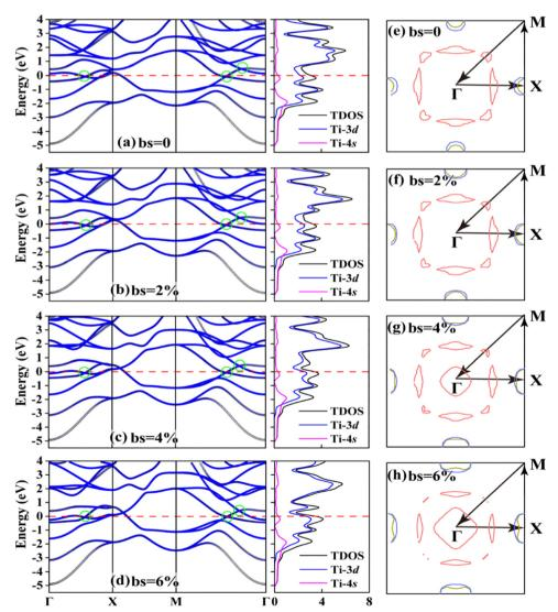
Fig. 4 (a-d) band structures (left), the projected and total density of states (DOS) (middle), and (e and f) the Fermi surface under different biaxial strains (bs): 0, 2%, 4%, and 6%. The bands crossing the Fermi energy are colored differently. The Ti-3d and Ti-4s orbital projected DOS and total DOS are colored in blue, pink and black. The evolution of the Dirac points is marked by green circles.
