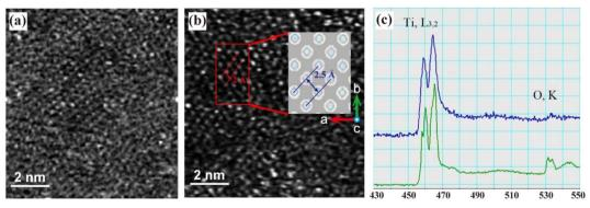
Fig. 1 (a) STEM image of the unirradiated suspended sample. (b) STEM image of the irradiated suspended sample. The inset shows the atomic configuration after irradiation. (c) The electron energy loss spectrum (EELS) before (in green) and after (in blue) e-beam irradiation. The highlighted Ti, L<sub>3,2</sub> and O, K edges are marked in the plot.
