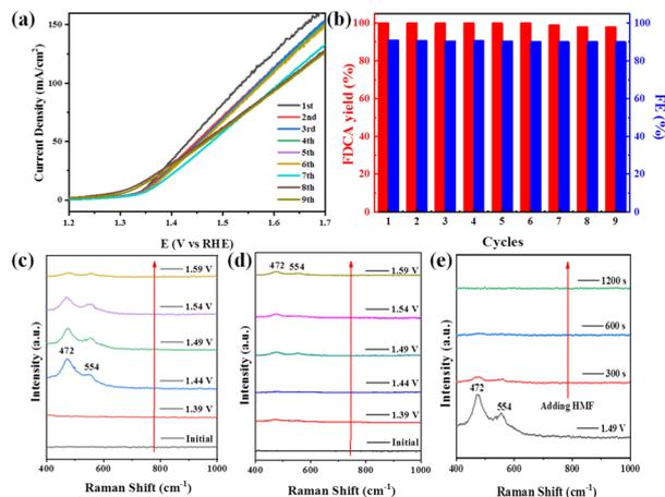
Fig. 4 (a) LSV curves of LN-400-P-350 in 1.0 M KOH with 10 mM HMF for nine successive cycles. (b) FDCA yields and FEs of LN-400-P-350 for nine successive cycles. (c) Potential-dependent *in situ* Raman spectra of LN-400-P-350 without HMF. (d) Potential-dependent *in situ* Raman spectra of LN-400-P-350 with HMF. (e) *In situ* Raman spectra at 1.49 V vs. RHE without HMF and after the addition of HMF.
