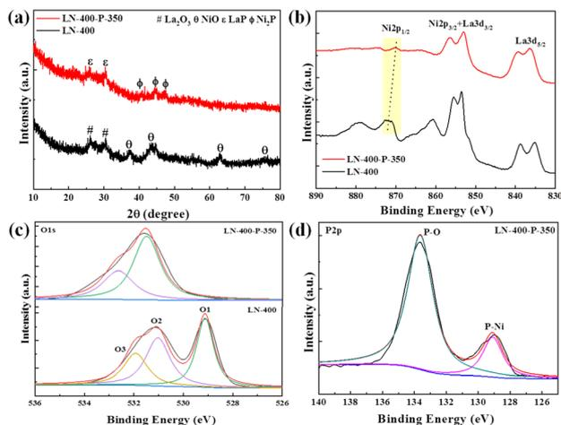
Fig. 2 (a) XRD patterns; (b) high resolution La 3d + Ni 2p spectra and (c) high resolution O 1s spectra of the LN-400 and LN-400-P-350 catalysts. (d) High resolution P 2p spectrum of the LN-400-P-350 catalyst.
