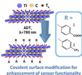
**Plasmon assisted  $\text{Ti}_3\text{C}_2\text{T}_x$  grafting and surface termination tuning for enhancement of flake stability and humidity sensing performance**
