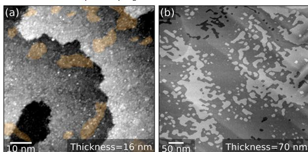
Fig. 5 LSMO(110) film grown at optimized conditions. (a)  $70 \times 70 \text{ nm}^2$  and (b)  $500 \times 500 \text{ nm}^2$  STM images of 16 nm-thick and of 70 nm-thick LSMO(110) films, respectively, grown onto a fishbone-reconstructed LSMO(110) surface at  $4.2 \times 10^{-2}$  mbar  $O_2$ . Both morphologies are atomically flat. At the atomic scale,  $(1 \times 1)$  patches are visible [orange in panel (a)].
