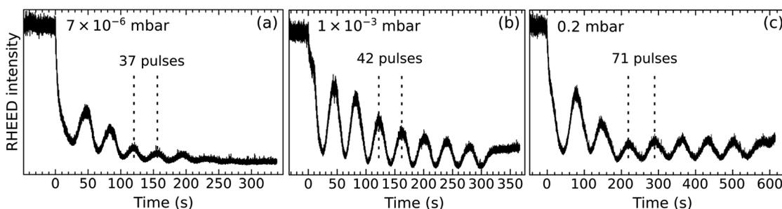
Fig. 2 RHEED oscillations during the growth of thin LSMO(110) films (≈2.5 nm thick) at different  $p_{\text{O}_2}$  (values indicated in the respective panels) and otherwise identical growth parameters (1 Hz, 1.9 J cm<sup>-2</sup>, 700 °C). Note that the data do not correspond to the same films as shown in Fig. 1.
