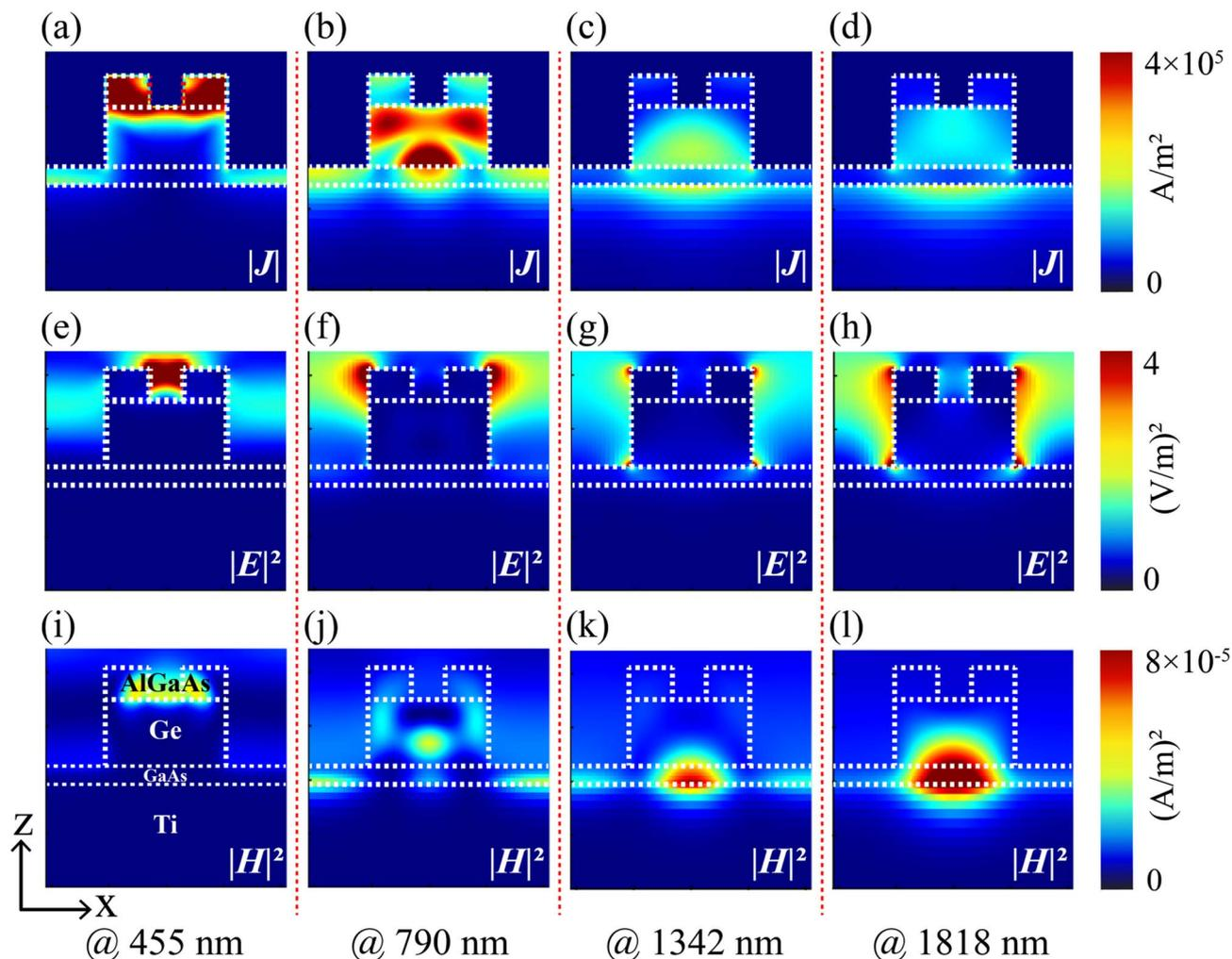
Fig. 3 Spatial  $xz$ -current density ( $|J|$ ) (a–d), -electric field ( $|E|^2$ ) (e–h), and -magnetic field ( $|H|^2$ ) (i–l) distributions for a unit cell under TM-polarized light at wavelengths of 455 nm, 790 nm, 1342 nm, and 1818 nm. The dotted lines depict the proposed double grating absorber structure.
