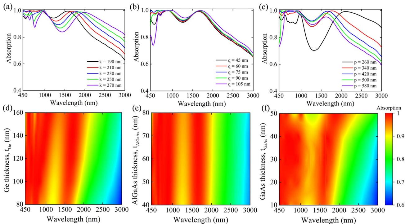
Fig. 4 Illustration of effects of the geometric parameters (a)  $k$ , (b)  $q$ , (c)  $p$ , (d)  $t_{\text{Ge}}$ , (e)  $t_{\text{AlGaAs}}$ , and (f)  $t_{\text{GaAs}}$  on absorption performances for TM-polarized light.
