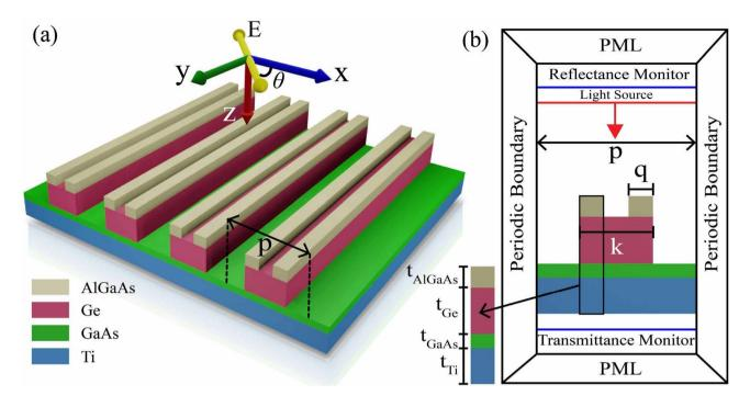
Fig. 1 (a) Illustration of a double-grating-based metamaterial absorber. A plane light wave was incident on the structure with an electric field along the z-direction where  $\theta$  is the polarization angle. (b) Cross-sectional view of the xz plane of our proposed absorber, where p=420 nm,  $t_{Ti}=200$  nm,  $t_{GaAs}=30$  nm,  $t_{GaAs}=3$
