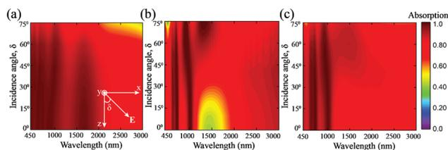
**Fig. 6** Color plot of calculated absorption spectra for different incidence angles for (a) TM, (b) TE, and (c) unpolarized light. The inset of (a) depicts the incidence angle,  $\delta$ , of a TM-polarized plane wave.
