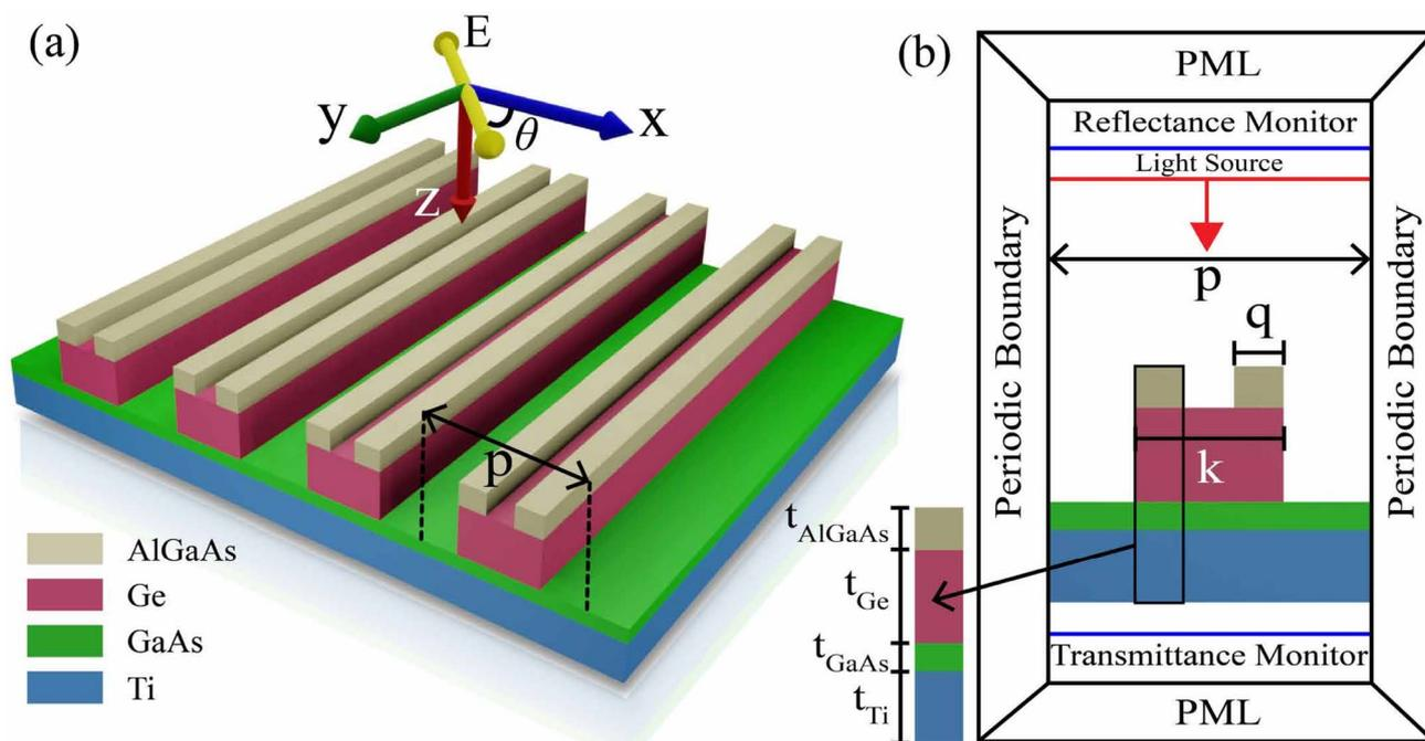
**Fig. 1** (a) Illustration of a double-grating-based metamaterial absorber. A plane light wave was incident on the structure with an electric field along the  $z$ -direction where  $\theta$  is the polarization angle. (b) Cross-sectional view of the  $xz$  plane of our proposed absorber, where  $p = 420$  nm,  $t_{\text{Ti}} = 200$  nm,  $t_{\text{GaAs}} = 30$  nm,  $k = 210$  nm,  $t_{\text{Ge}} = 120$  nm,  $q = 75$  nm, and  $t_{\text{AlGaAs}} = 60$  nm.
