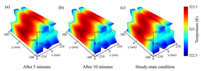
Fig. 8 Evolution of heat temperature profiles of the proposed metamaterial double-grating structure under transient response after (a) 5 minutes and (b) 10 minutes. (c) Evolution of heat temperature profiles of the proposed metamaterial double-grating structure under steady-state conditions
