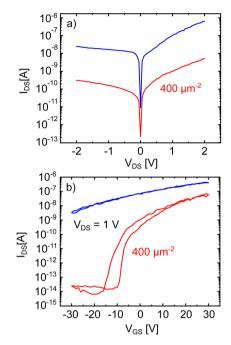
Fig. 2 (a) Output and (b) transfer characteristics of a MoS $_2$  FET before (blue) and after (red) irradiation with Xe $^{30+}$  ions with a fluence of 400 ions/ $\mu$ m $^2$ .
