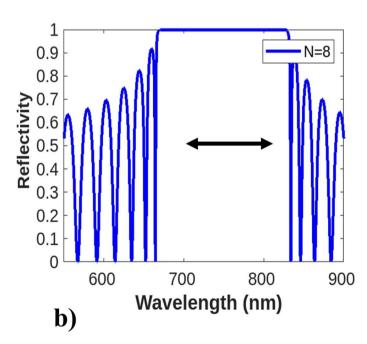
Fig. 8 Design and optical phenomena of a photonic crystal. (a) Shows the design of photonic crystals with a different arrangement of dielectric layers having a low and high refractive index, photonic crystal-light interaction, and how light behaves. (b) Shows a Bragg reflector with broad photonic band gap reflection spectra. This figure has been reproduced from ref. 109 with permission from IEEE, copyright 2002.
