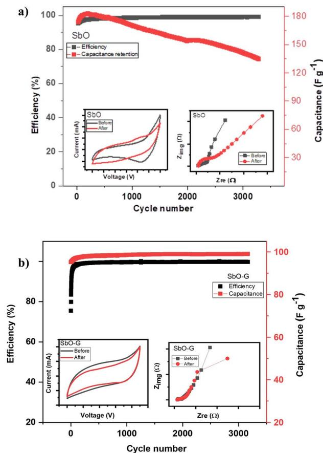
Fig. 9 Cycling stability of (a) AC//SbO and (b) AC//SbO-G supercapacitor over 4500 cycles in 1 M  $\text{Li}_2\text{SO}_4$ . The inset in (a and b) is the CV plot ( $50 \text{ mV s}^{-1}$ ) and EIS plot before and after cycling.
