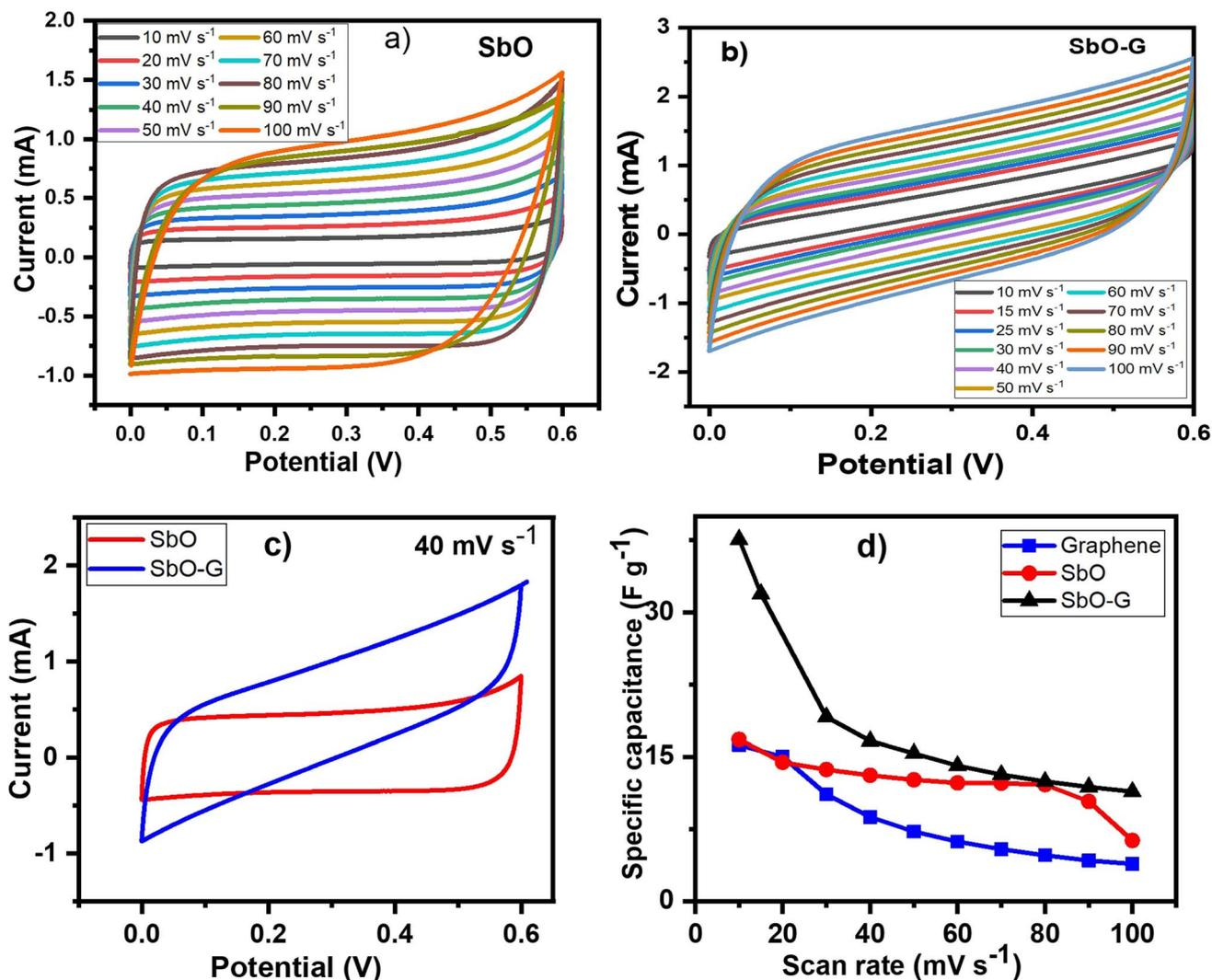
Fig. 4 SbO and SbO-G: (a and b) CV plots at different scan rates, (c) CV plots comparing their voltammograms at  $40 \text{ mV s}^{-1}$  scan rate, (d) their specific capacitances at different scan rates. All analysis was done in  $1 \text{ M Li}_2\text{SO}_4$  electrolyte.
