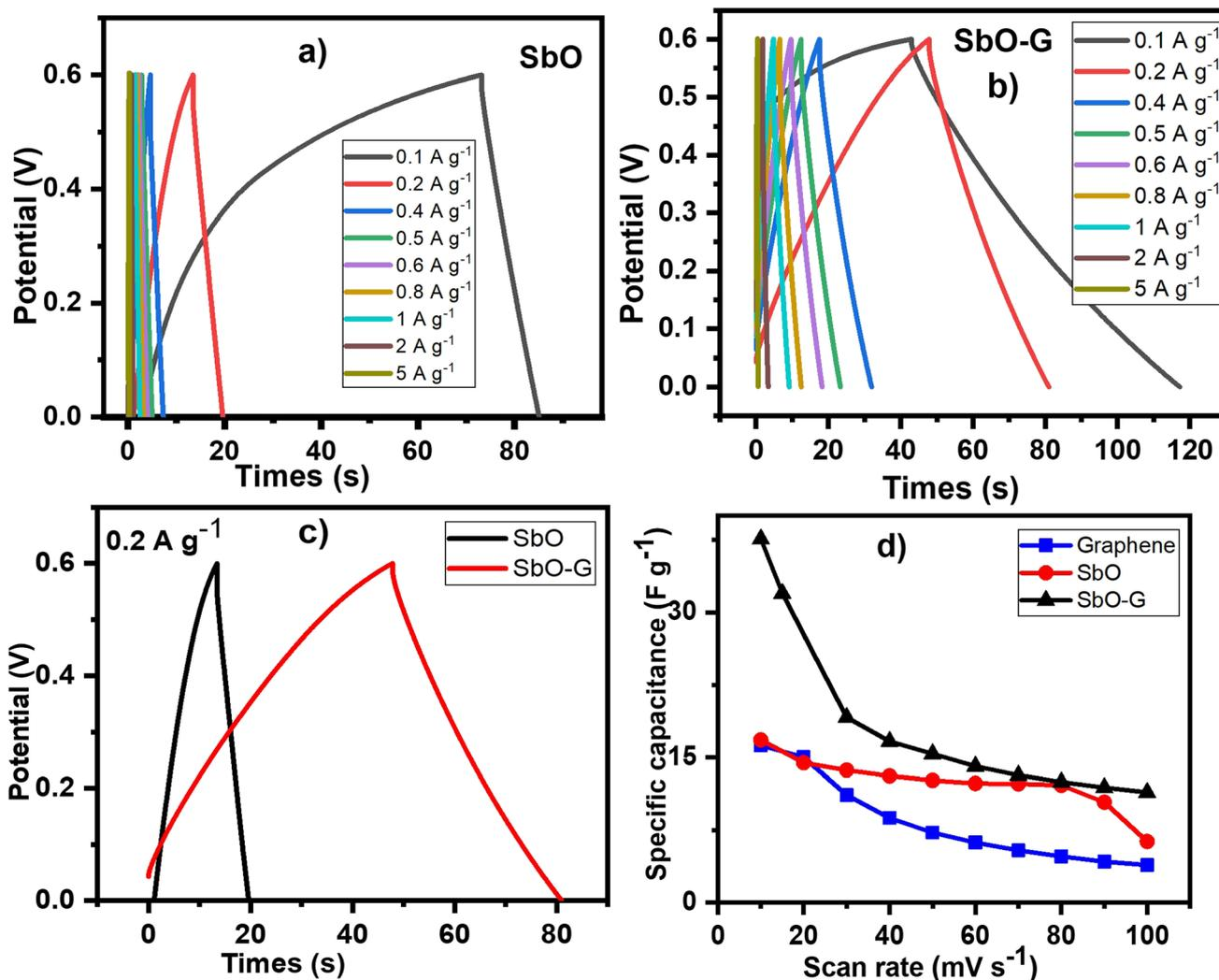
Fig. 5 SbO and SbO-G: (a and b) GCD plots at different current densities, (c) GCD plots comparing their charge and discharge profile at 0.2 A g<sup>-1</sup> current density, (d) is their specific capacitance at different current densities. All analysis was done in 1 M Li<sub>2</sub>SO<sub>4</sub> electrolyte.
