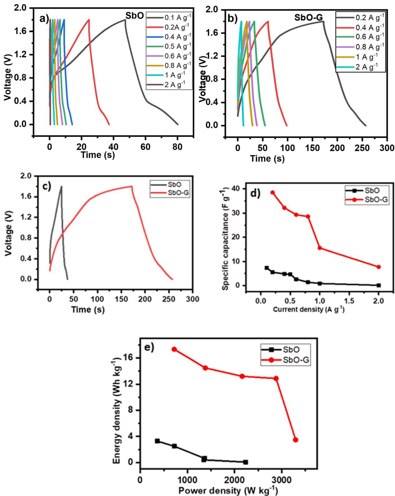
Fig. 7 AC//SbO and AC//SbO-G: (a and b) GCD plots at different current densities, (c) GCD plots comparing their charge and discharge profile at 0.2 A g<sup>-1</sup> current density, (d) relationship between specific capacitance and current density (e) is the Ragone plot. All analysis was done in 1 M Li<sub>2</sub>SO<sub>4</sub> electrolyte.
