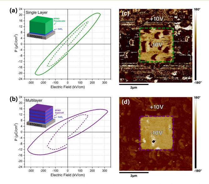
Fig. 5 Ferroelectric property characterization by (a and b) P-E loops and (c and d) PFM area scans. The (a and c) single layer and (b and d) multilayer samples are characterized.
