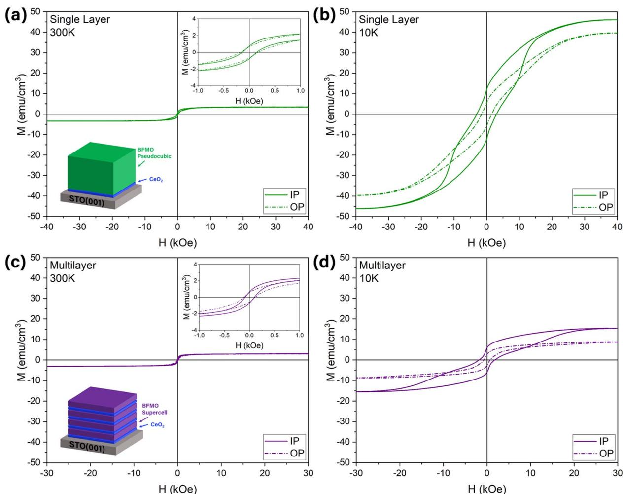
Fig. 4 Magnetic property characterization of (a and b) the thick single layer and (c and d) multilayer films at (a and c) 300 K and (b and d) 10 K. In-plane and out-of-plane data is included for each sample and measurement condition.
