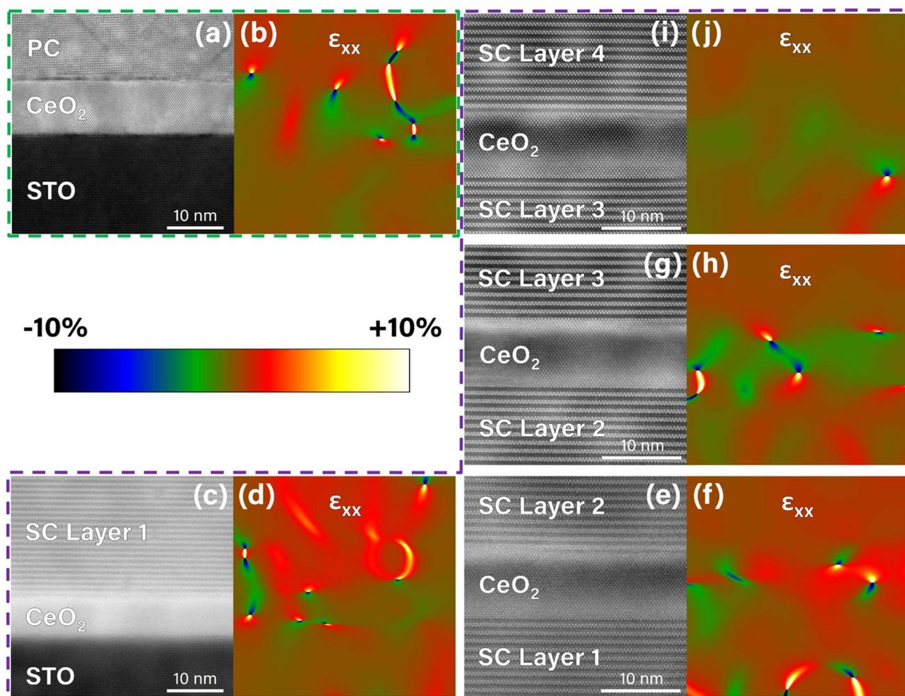
Fig. 3 Geometric phase analysis strain images of (a and b) the thick single layer and (c–j) multilayer films. The HR-STEM image of each area is shown with the corresponding in-plane strain image,  $\epsilon_{xx}$ , where the spatial dimensions and physical area are the same. A color scale bar representing the strain is provided for the strain map images, which all have identical strain scales of  $-10\%$  to  $+10\%$ .
