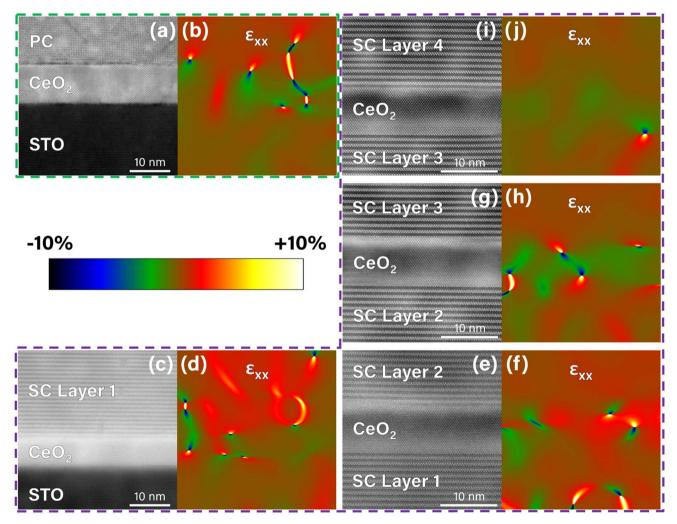
Fig. 3 Geometric phase analysis strain images of (a and b) the thick single layer and (c–j) multilayer films. The HR-STEM image of each area is shown with the corresponding in-plane strain image,  $\varepsilon_{xx}$ , where the spatial dimensions and physical area are the same. A color scale bar representing the strain is provided for the strain map images, which all have identical strain scales of -10% to +10%.
