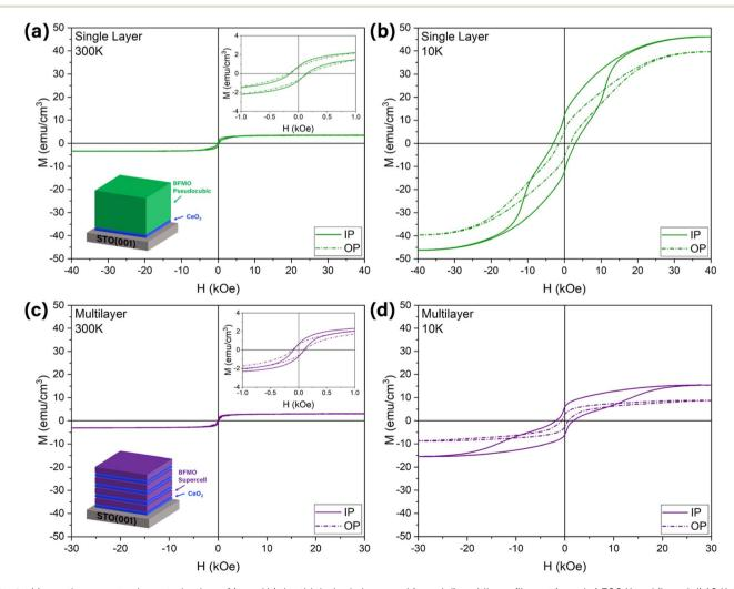
Fig. 4 Magnetic property characterization of (a and b) the thick single layer and (c and d) multilayer films at (a and c) 300 K and (b and d) 10 K. Inplane and out-of-plane data is included for each sample and measurement condition.
