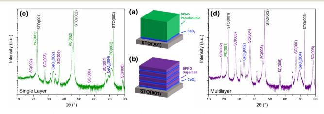
Fig. 1 Film structure of (a and c) thick single layer and (b and d) multilayer films. (a and b) Schematic drawings and (c and d) XRD data are shown for each.
