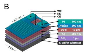
Fig. 4 (A) Electrochemical methane sensing using IL-based electrolytes. CO<sub>2</sub> generated by successive methane oxidation on the WE, and active oxygen species were used as an internal standard. Adapted with permission from ref. 162 Copyright 2014 Royal Society of Chemistry. (B) Scheme showing a multilayered electrochemical device based on solid-state electrolyte Nafion for methane sensing. Reprinted with permission from ref. 161 Copyright 2018 American Chemical Society.
