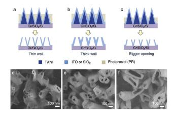
(a)-(c) Schematic diagram illustrating methods for controlling the wall thickness and opening size of the nanotube arrays. (d)-(f) SEM images of the resulting vertical nanotube arrays for (a)-(c), respectively
