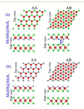
Fig. 2 Atomic structures of (a) MoSH@MoS2 and (b) MoHS@MoS2 heterostructures for different stacking patterns of AA and AB.
