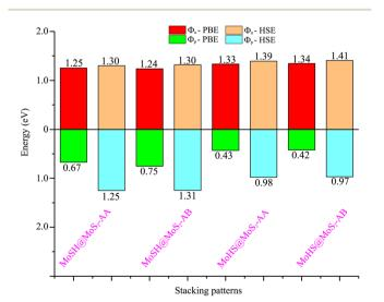
Fig. 4 Calculated SBHs of the heterostructures between MoSH and  $MoS_2$  monolayers for different configurations using PBE and HSE functionals.
