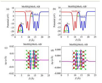
Fig. 5 Electrostatic potential of (a) MoSH@MoS $_2$  and (b) MoHS@MoS $_2$  heterostructures for the AB stacking pattern. 2D planar-averaged charge density differences of (c) MoSH@MoS $_2$  and (d) MoHS@MoS $_2$  heterostructures for the AB stacking pattern. The yellow regions represent areas of charge accumulation, while the cyan regions indicate charge depletion.
