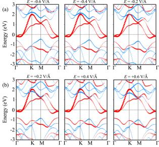
Fig. 7 Projected band structures of the MoSH@MoS<sub>2</sub> heterostructure for the AB pattern for different strengths of (a) negative and (b) positive electric fields. Red and green lines represent the contributions of MoSH and MoS<sub>2</sub> layers, respectively.
