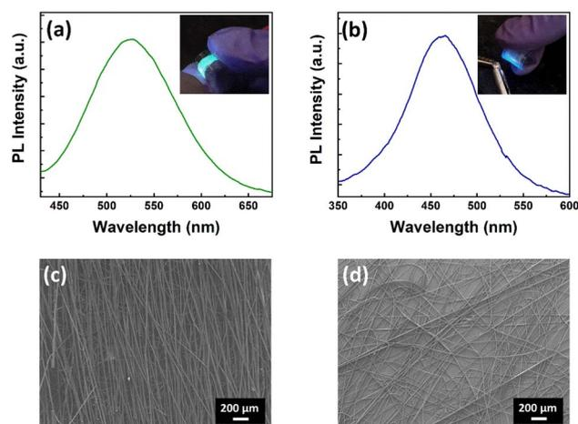
Fig. 8 PL spectra of (a)  $\text{Cs}_3\text{Cu}_2\text{Cl}_5$ @PMMA fibers and (b)  $\text{Cs}_3\text{Cu}_2\text{Br}_{2.5}\text{I}_{2.5}$ @PMMA fibers coated on PET substrates. Insets of (a) and (b) show photographic images of fibers coated on PET substrates and placed under a UV lamp. LR-FESEM images of (c)  $\text{Cs}_3\text{Cu}_2\text{Cl}_5$ @PMMA fibers and (d)  $\text{Cs}_3\text{Cu}_2\text{Br}_{2.5}\text{I}_{2.5}$ @PMMA fibers coated on PET substrates.
